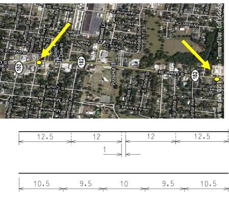
Figure 4 LA 182 layout and lane configuration before and after the project (dimensions are in feet)
