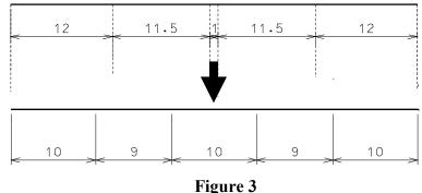
LA 3025 layout and lane configuration before and after the project (dimensions are in feet)
