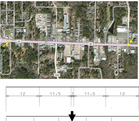
Figure 5 LA 28 layout and lane configuration before and after the project (dimensions are in feet)
