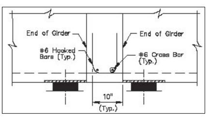
Detail of reinforcement placement at positive moment connection (section view) (NCHRP 519 Report)
