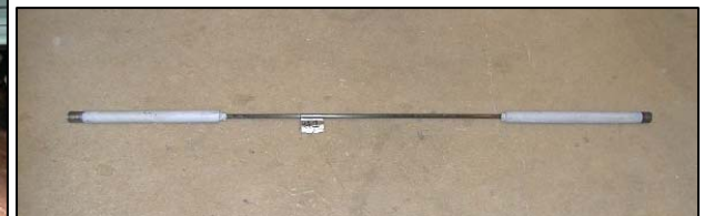
A sample FRP rod used for post-tensioning
