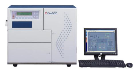
Figure 2 Tosoh EcoSEC high performance GPC system (HLC-8320GPC) from LA DOTD Materials Laboratory
