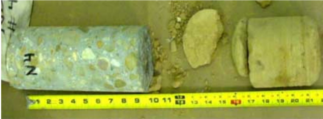
Figure 42 Concrete core with soil cement specimen
