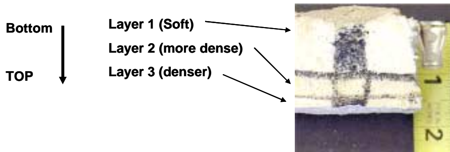
Figure 26 Polyurethane in trenched area (Area 3 Slab 74)
