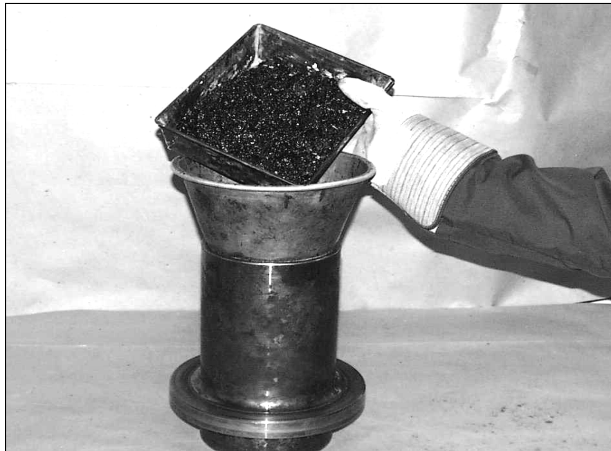
Figure 14 Placement of loose mix on top of a compacted bottom half
