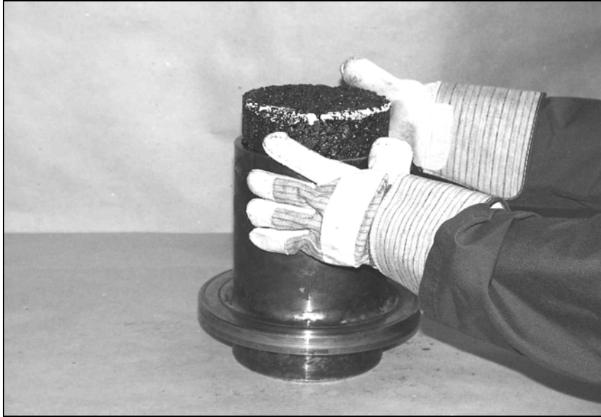
Figure 13 Placement of the compacted bottom half of a sample in mold
