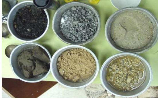
Figure 4 Dry-out tests of different backfill materials
