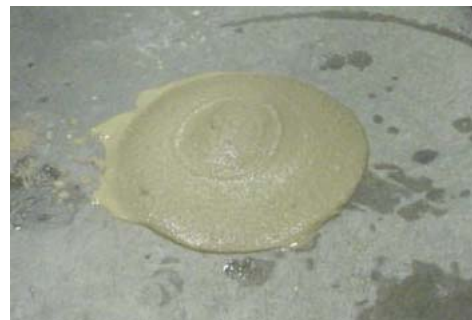
Figure 19 3×6 inches-open-ended cylinder flow consistency test
