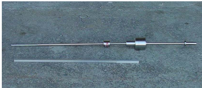
Figure 6 Dynamic cone penetration (DCP) device
