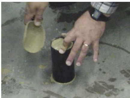
Figure 19 3×6 inches-open-ended cylinder flow consistency test
