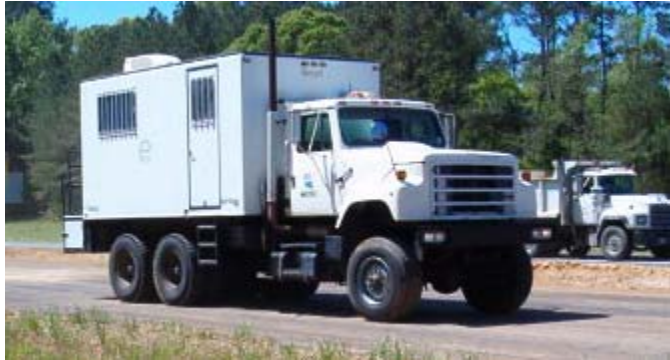
Figure 14 Twenty-ton LTRC cone truck
