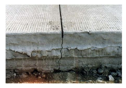
(b) Controlled crack developed underneath the narrow transverse contraction joint at test section S2 established using the early entry dry saw cut method
