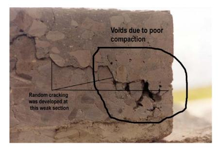
(b) Poor construction practice resulted in development of random cracking within the concrete pavement slab
