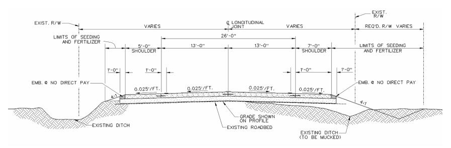
Figure 11 Typical section of the JPCP constructed at Northline Road
