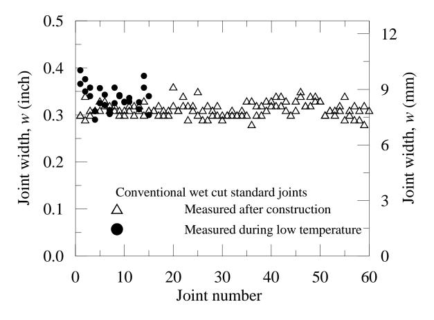
Figure 28 Results of the measurements of joints dimensions after construction and during the extreme low temperature season, conventional wet cut standard joints
