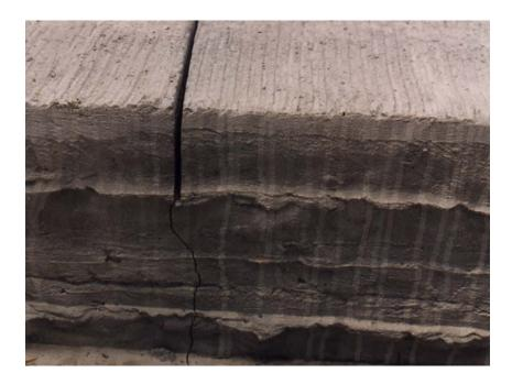
(a) Controlled crack developed underneath the standard contraction joint at test section S1 established using the conventional wet saw cut method
