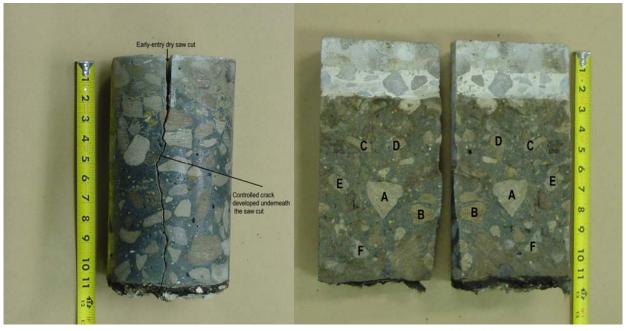
(a) Crack propagation underneath the early entry dry saw cut
