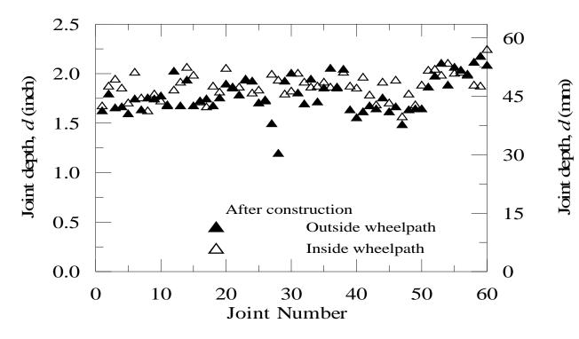
Figure 30 Results of the joint depth measurements, conventional wet cut standard joints
