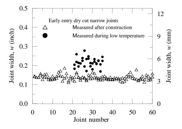
Figure 27 Results of the measurements of joints dimensions after construction and during the extreme low temperature season, early entry dry narrow joints
