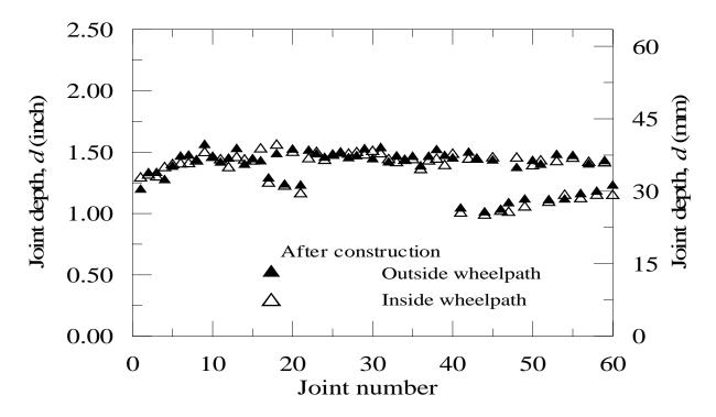
Figure 29 Results of the joint depth measurements, early entry dry cut narrow joints
