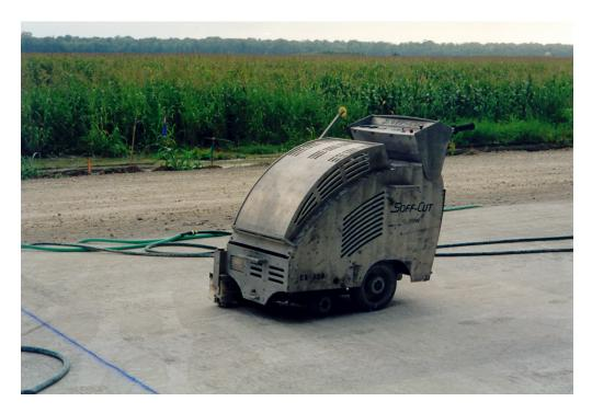
Figure 13 The early entry dry cut saw used in creating the narrow joints at test section S2
