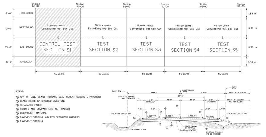
Figure 15 The standard and narrow joint test sections at Northline Road
