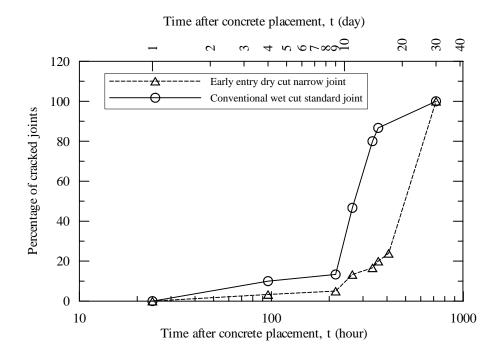
Figure 19 Comparison of the rate of propagation of controlled cracking within the investigated joint cut methods
