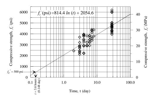
Figure 16 Compressive strength of the cement-slag concrete mix used for the pavement construction
