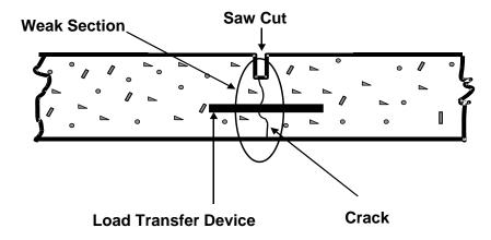
Figure 1 The elements of transverse contraction joints in plain jointed concrete pavements
