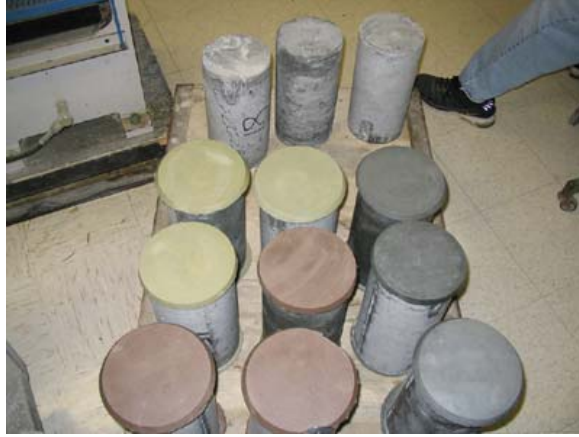
Figure 4 Concrete specimens with capping ready to be tested in compression, the specimens in the back were tested using unbonded pads
