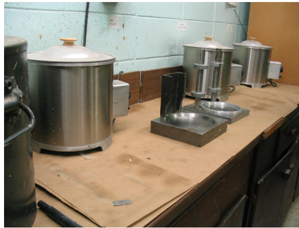
Figure 3 Individual melting pots were used for each capping compound to eliminate contamination, capping devices are also shown
