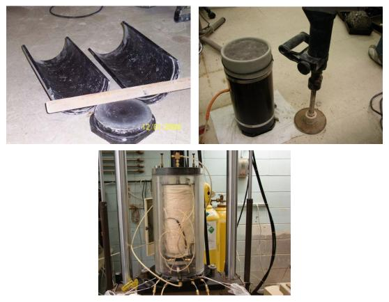
Figure 10: Compaction of RLT test samples
