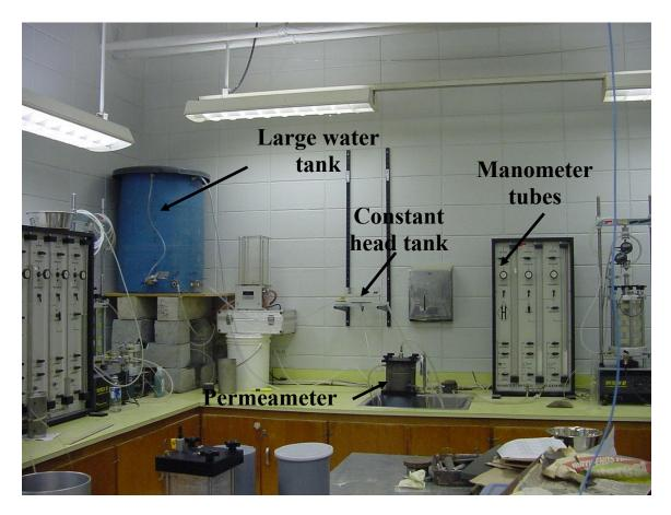
Figure 7: Picture of setup for constant-head hydraulic conductivity test
