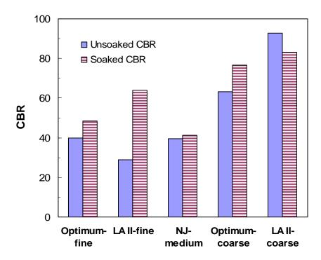
Figure 18: CBRs at 0.2 inches penetration for Mexican limestone at different gradations
