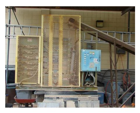
Figure 5: Picture of shaker machine for sorting unbound aggregate
