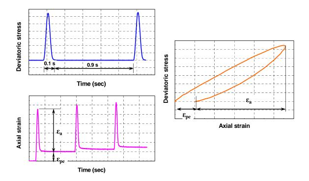
Figure 21: Typical results from a RLT test
