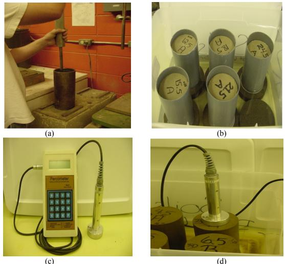
Figure 8: Tube suction test procedure: (a) sample compaction; (b) samples ready for TS test; (c) capacitance probe; and (d) taking readings
