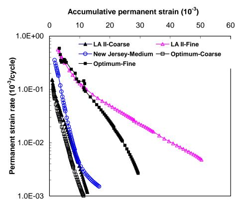
Figure 24: Variation of permanent strain rate with accumulative permanent strain for Mexican limestone specimens with different gradations
