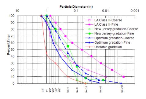
Figure 12: Particle size gradations of tested specimens
