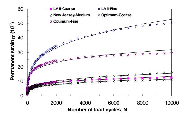
Figure 23: Variation of permanent deformation with number of load cycles for Mexican limestone specimens with different gradations
