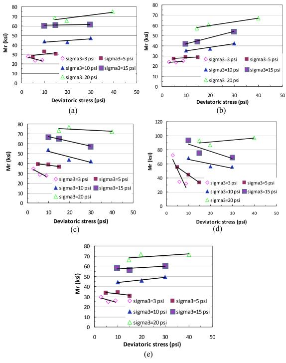
Figure 22: Resilient moduli of Mexican Limestone at various gradations at corresponding optimum compaction conditions: (a) LA II-coarse; (b) LA II-fine; (c) NJ-medium; (d) Optimum-coarse; and (e) Optimum-fine
