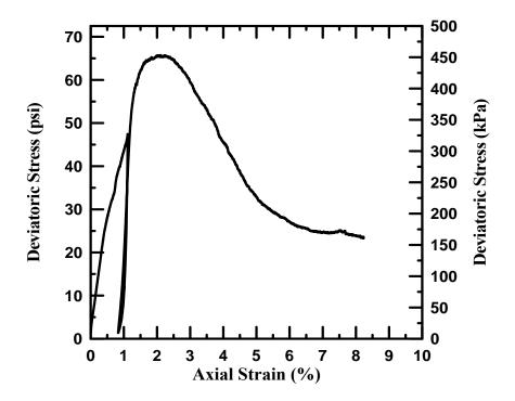
Figure 20: Results of Monotonic Loading Triaxial Test
