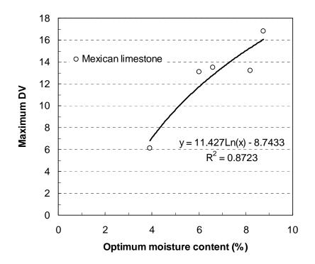
Figure 16: Correlation between maximum DV values and optimum moisture contents determined from Standard Proctor tests for Mexican limestone with different gradations
