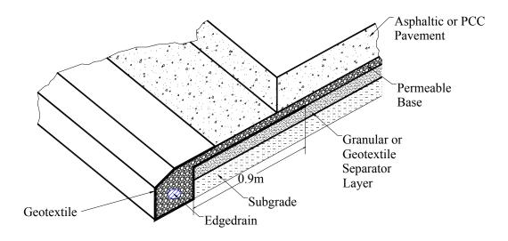
Figure 1: Components of a subsurface drainage system (after [1])
