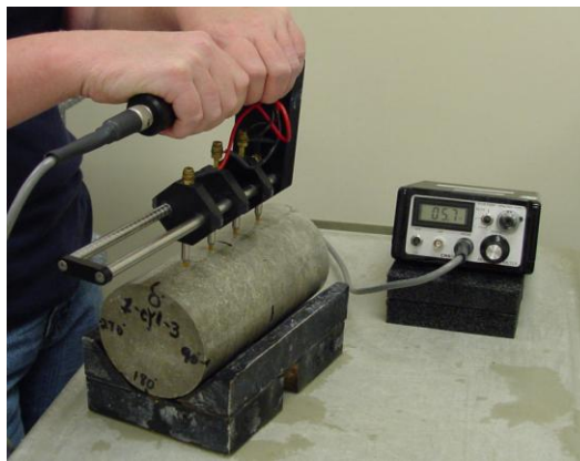
Figure 3 Surface resistivity test being conducted
