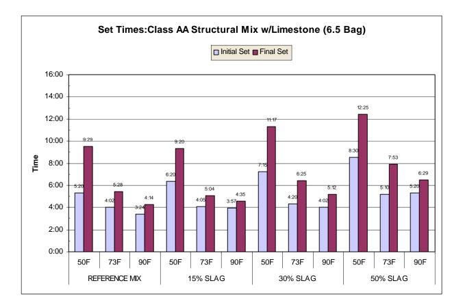
As compared to the previous study on grade-120 GGBFS, there were no distinguishable trends between the two grades of GGBFS or the substitution amounts of GGBFS relating to set times. Differences were noticed in reference mixes along with mixes containing GGBFS. As evident in the following two graphs, set times for GGBFS concrete increases in proportion to the substitution
