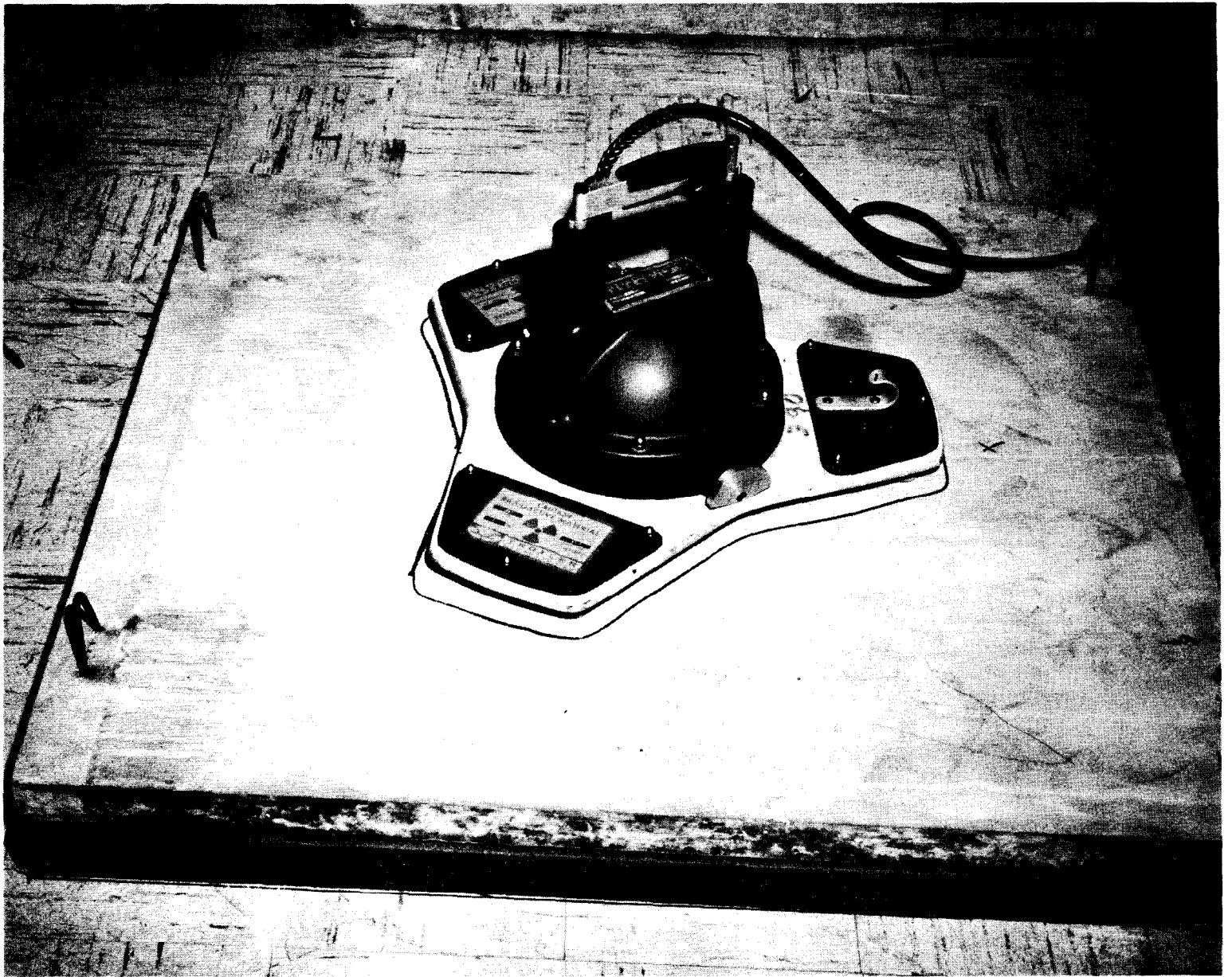
Figure 7 - Photograph of the Nuclear Device Testing a Concrete Slab Overlaying a 2 Inch Piece of Styrofoam
