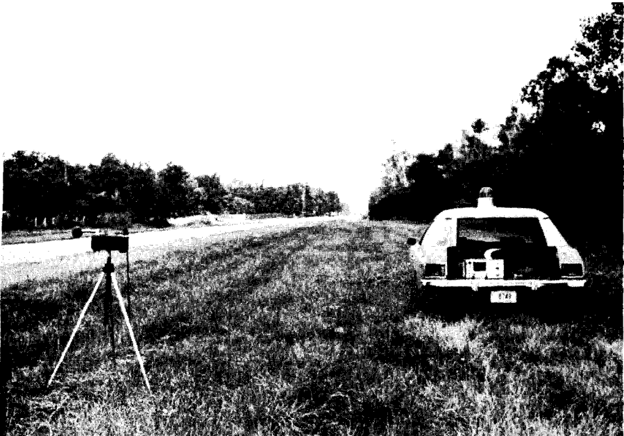
Typical Field Set Up Using Graphic Level Recording Equipment FIGURE 3
