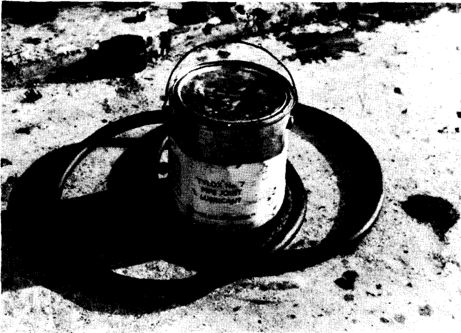
Figure 6 "O" Rings and Pipe Joint Lubricant for Helical Pipe with Annular Ends
