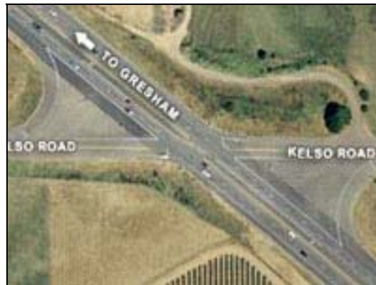
Figure 5.3: Intersection skew angle
