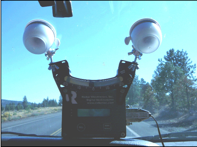
Figure 4.6: Ball-bank indicators mounted in test vehicle
