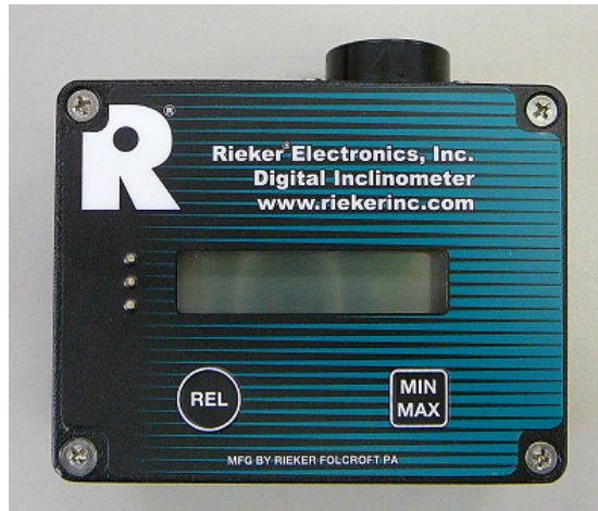
Figure 4.4: Electronic “ball-bank” indicator
