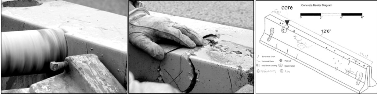
Figure 3.1: Example of core sample extraction. This core (001) was taken from barrier 001 in Ladd Canyon
