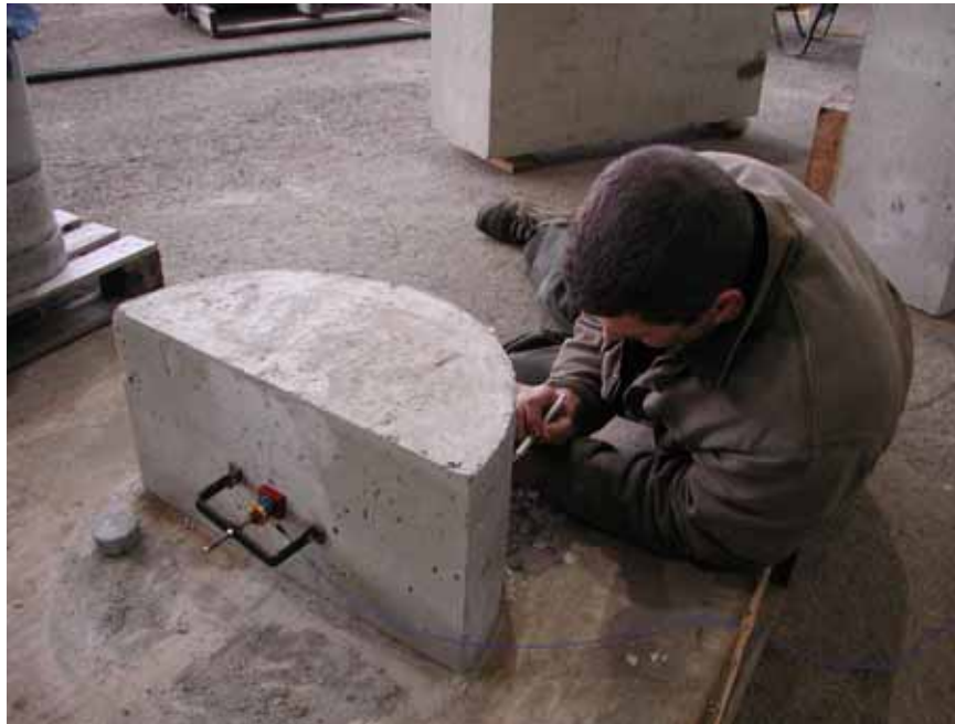
Figure 5.8: Semi-circular specimen, experimental setup
