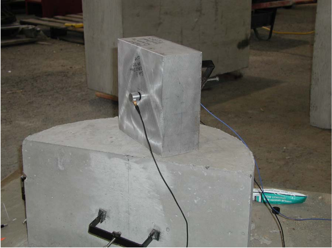
Figure 3.2: Calibration test on an aluminum block.
