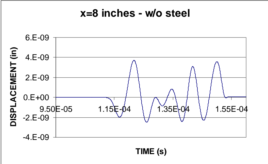
Figure B.9: FEA results for the un-reinforced concrete block at position x=8 inches
