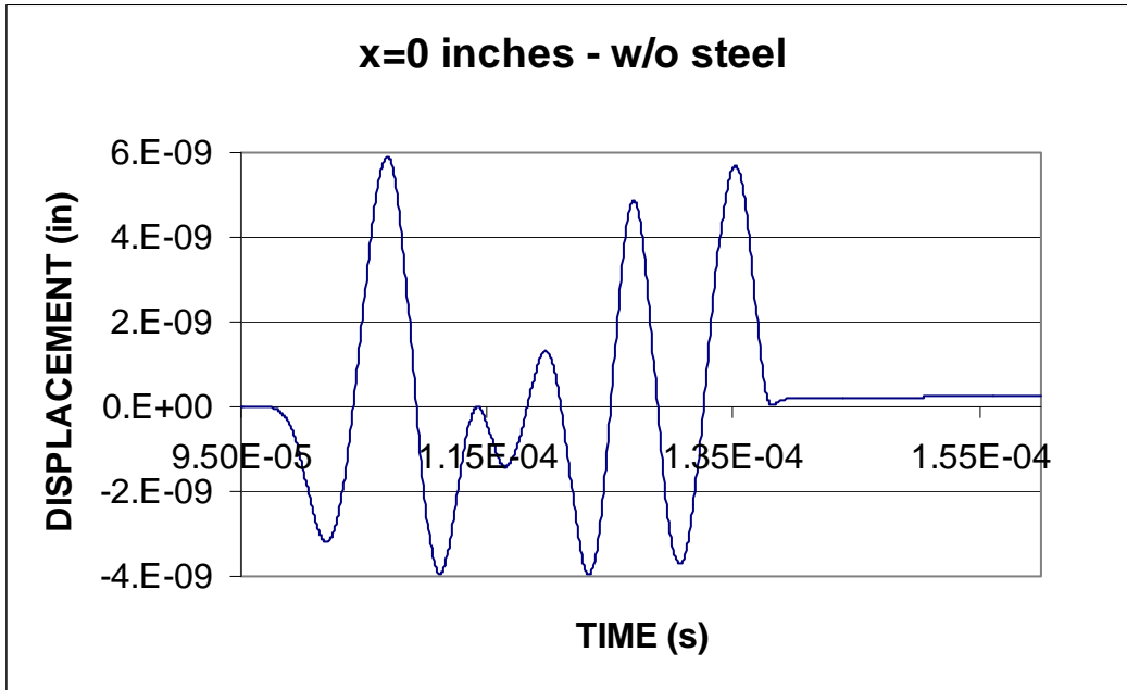
Figure B.1: FEA results for the un-reinforced concrete block at position x=0 inches
