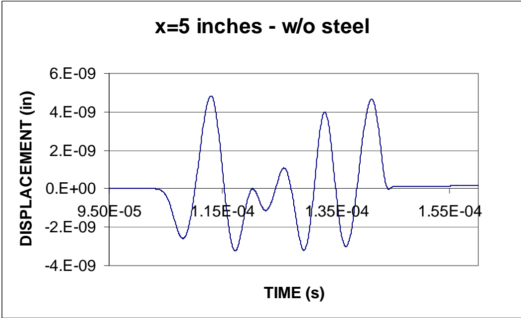
Figure B.6: FEA results for the un-reinforced concrete block at position x=5 inches
