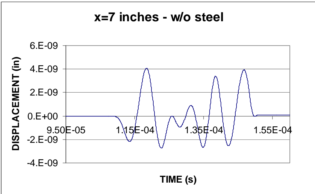
Figure B.8: FEA results for the un-reinforced concrete block at position x=7 inches
