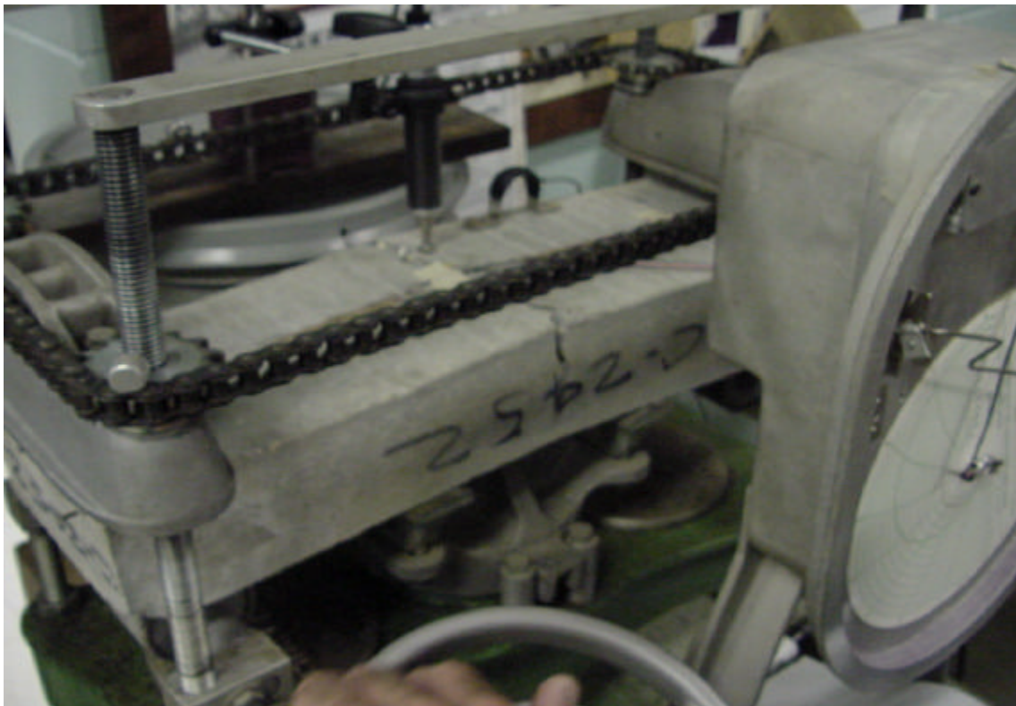
Figure 17 The cracking appears at the middle span of the fourth beam
