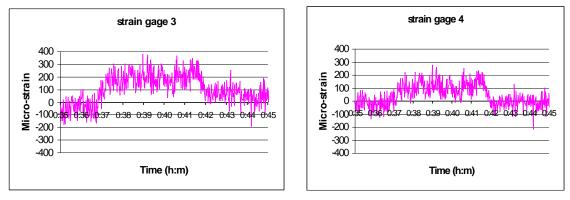
Figure 19 Actual results for strain gauges 1-4 (midspan of girders)
