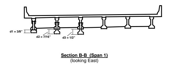
Figure 26 Deflection results for girders at midspan (span 1)
