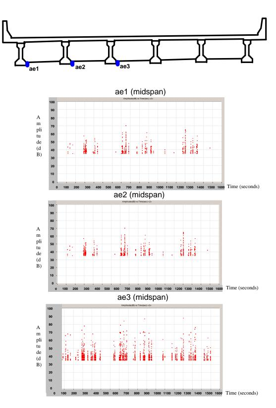
Figure 29 Amplitude vs. time – Traffic Scan 2
