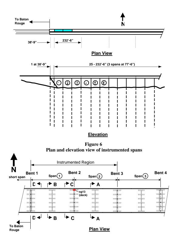
Figure 7 Plan view of instrumented portion of the bridge
