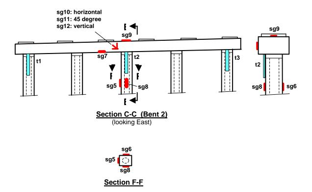
Figure 10 Strain gauge and target numbering (bent 2)
