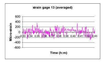
Figure 23 Actual and smoothed results for strain gauge 13 (in deck over bent 2)
