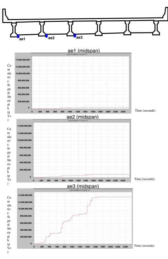
Figure 30 Cumulative Strength Signal - Traffic Scan 2
