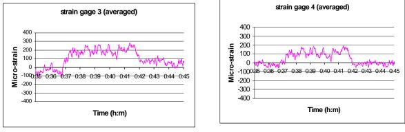
Figure 20 Smoothed results for strain gauges 1-4 (midspan of girders)
