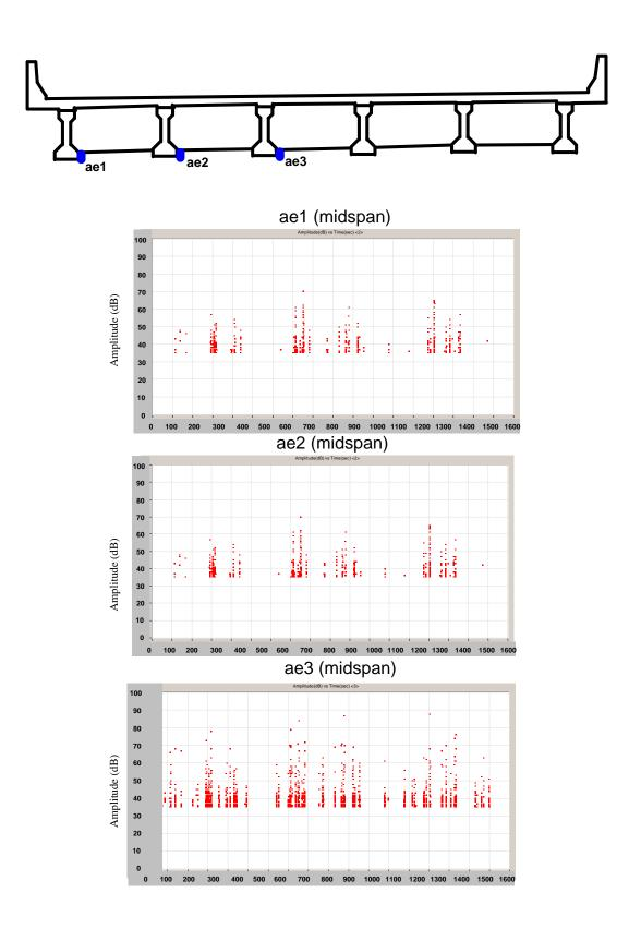
Figure 28 Amplitude vs. time - Traffic Scan 1
