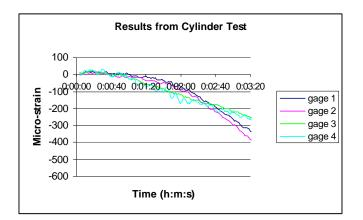
Figure 14 Strain results from concrete cylinder test
