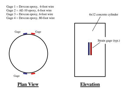
Figure 13 Concrete cylinder test for validation of strain measurements
