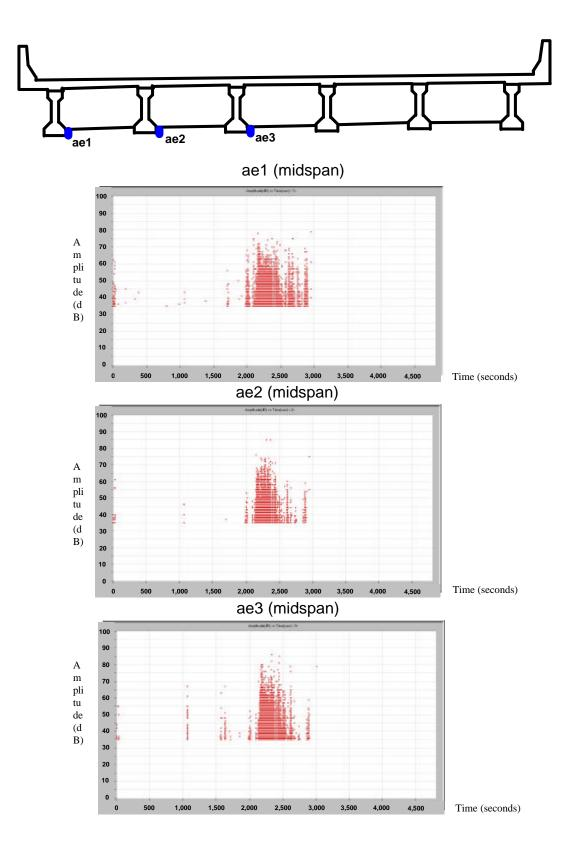
Figure 31 Amplitude vs. Time - Overload 2
