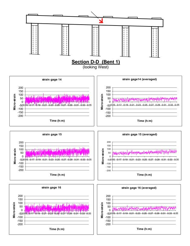
Figure 24 Actual and smoothed results for strain gauges 14, 15, and 16
