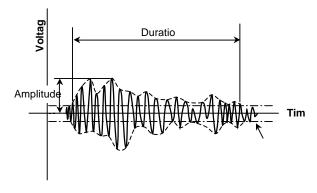
Figure 27 Schematic of Acoustic emission hit recorded by resonant sensor
