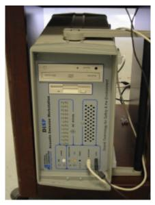
Figure 16 Photograph of Portable acoustic Emission Monitoring System
