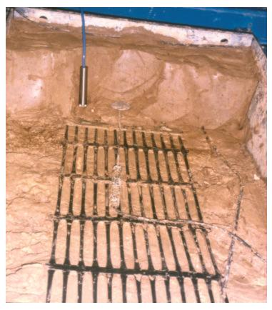
Figure 19 View of the geogrid specimen in the pullout box
