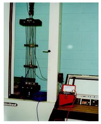
Figure 9 View of the instrumented geogrid specimen in the extension test
