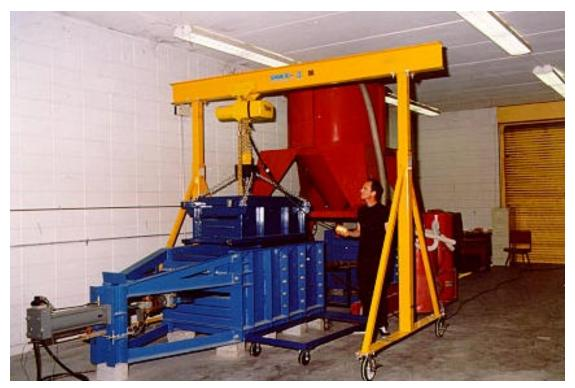
Figure 18 Loading the pullout box inside the hydraulic loading frame
