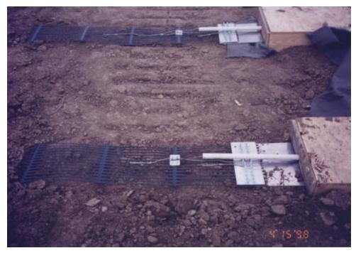
Figure 27 View of the instrumentation in geogrid UX-1500
