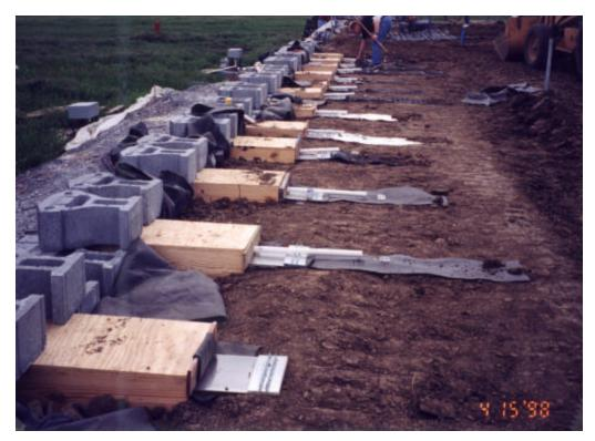
Figure 24 View of the pullout boxes inside the test wall
