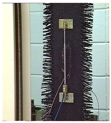
Figure 14 Calibration of strain gauges in the woven geotextiles
