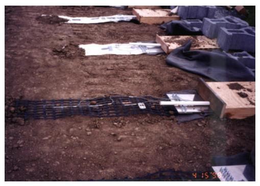
Figure 28 View of the instrumentation in geogrid Stratagrid-500
