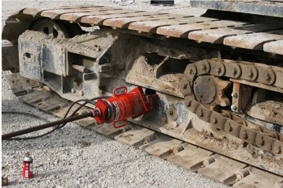
Figure 32: Loading Mechanism for the Pile with Steel Plate
