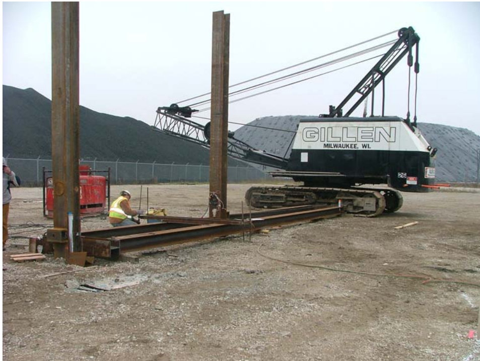
Figure 41: Loading Mechanism (Pile with Concrete Pier Test)
