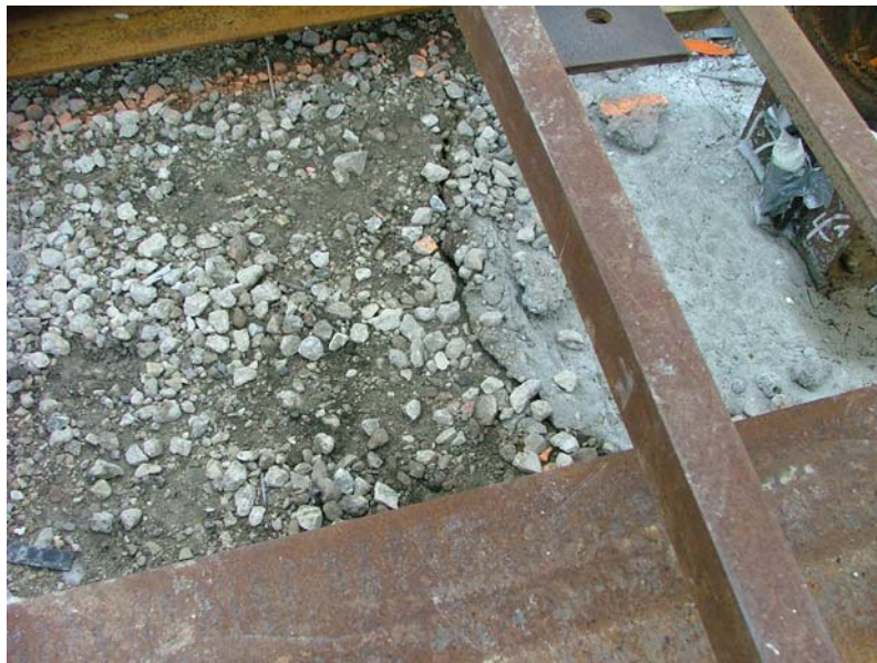
Figure 46: Gap at 556 kN-667 kN (125,000 lb-150,000 lb)
