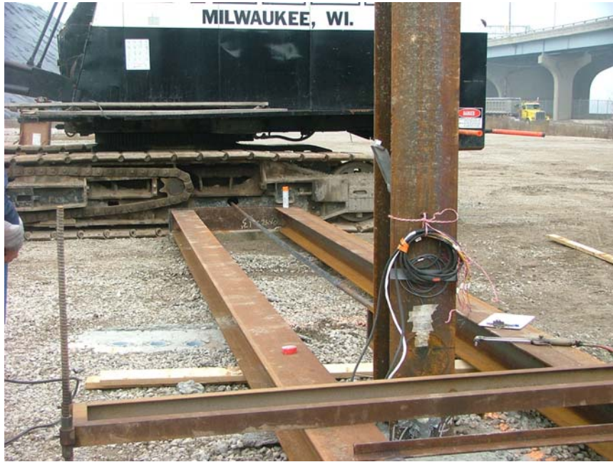
Figure 42: Loading Mechanism (Pile with Concrete Pier Test)
