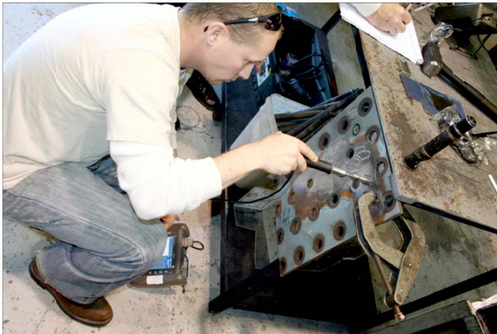
Figure 11. Performing Ultrasonic Hardness Testing on Defective A 514 Steel in Vertical Test Orientation by Pressing Probe into the Steel.
