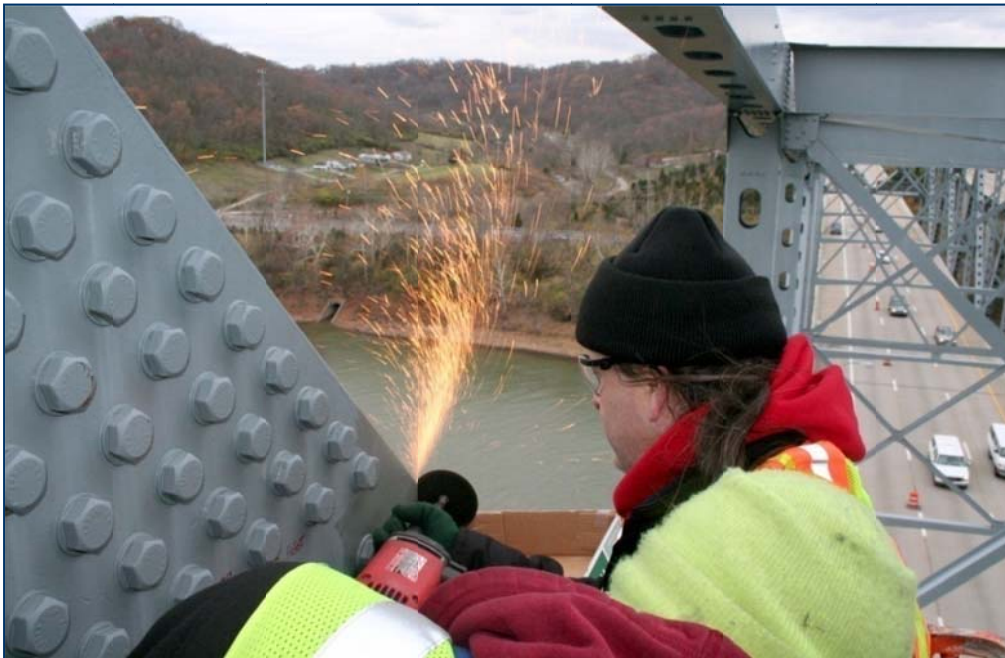
Figure 25. IMR Technician Cutting Corner Specimen from A 514 Steel Splice Plate that Provided Low Hardness Readings.
