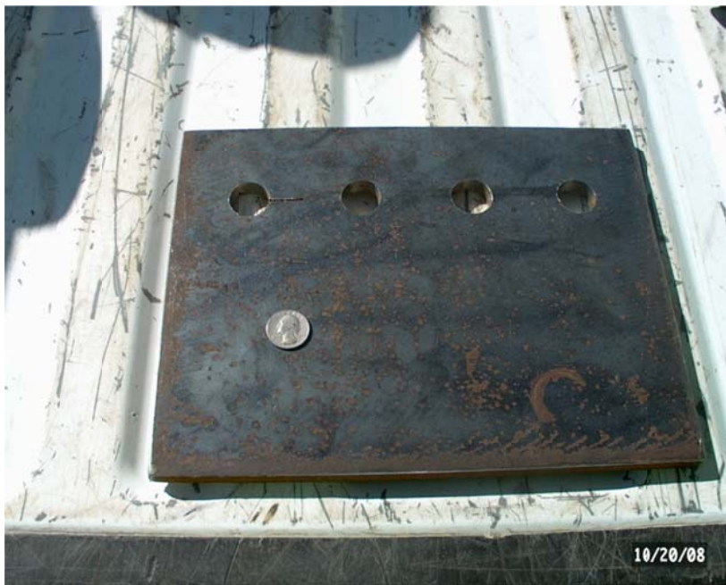
Figure 21. Special Calibration Plate Used for Nondestructive Evaluation of 1/2" Splice Plates at Tower (U16) Locations on the Two I-275 Bridges.
