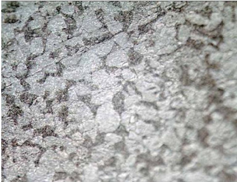
Figure 24. Replica of A 514 Steel Showing Ferritic-Fine Carbide Microstructure (~600X).
