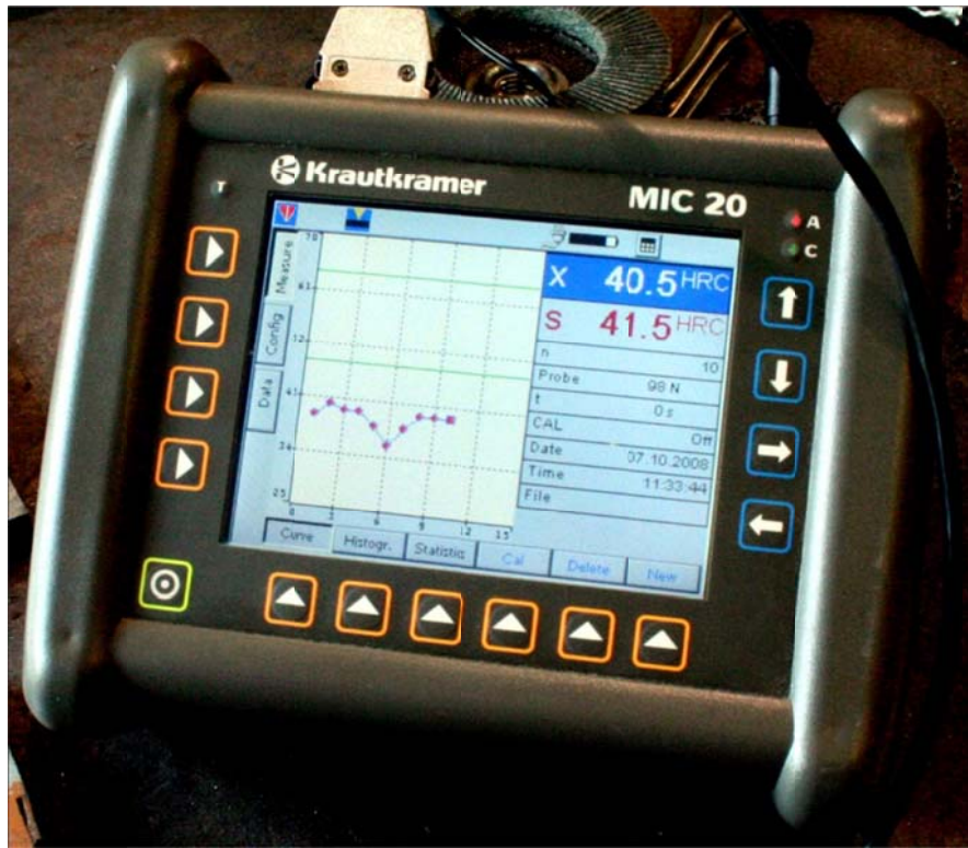
Figure 12. Screen Read-Out of GE/Krautkramer MIC 20 for Tests on Defective Steel. Individual Test Values are indicated by Red Numbers (e.g. 41.5 HRC) in Upper Right Corner of Screen. The Running Average of a Series of Tests is indicated by White Numbers above (e.g. 40.5 HRC).
