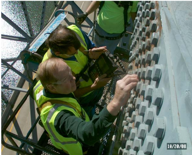
Figure 22. HTT NDE Supervisor Performing Ultrasonic Shear Wave Inspections on a 1/2" Splice Plate on the Downstream Truss of the Westbound Bridge.
