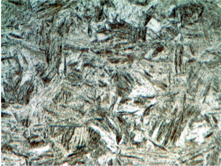
Figure 6. Microstructure of Improperly Tempered A 514 Steel from Cracked Splice Plates (1000X Magnification). Etchant: 2% Nital.
