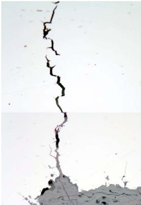
Figure 7. Photomicrograph montage of Intergranular Cracking Emanating from Corrosion Pit in A Cracked Splice Plate (250X Magnification). As - Polished.
