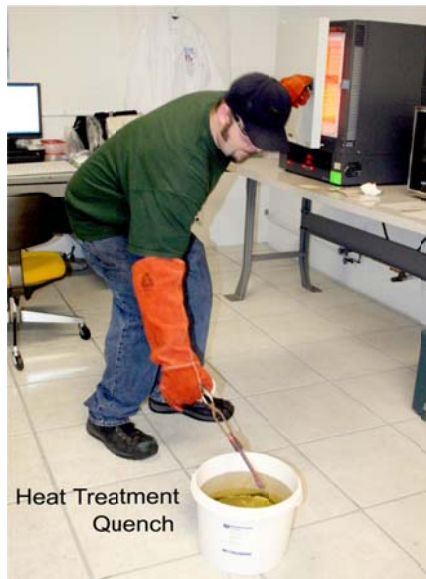
Figure 9 A. Quenching A 514 Pieces after Re-Heating (and Prior to Re-Tempering) and B. Charpy Impact Testing Re-Tempered Pieces to Investigate the Relationship between Indentation Hardness and Impact Toughness.
