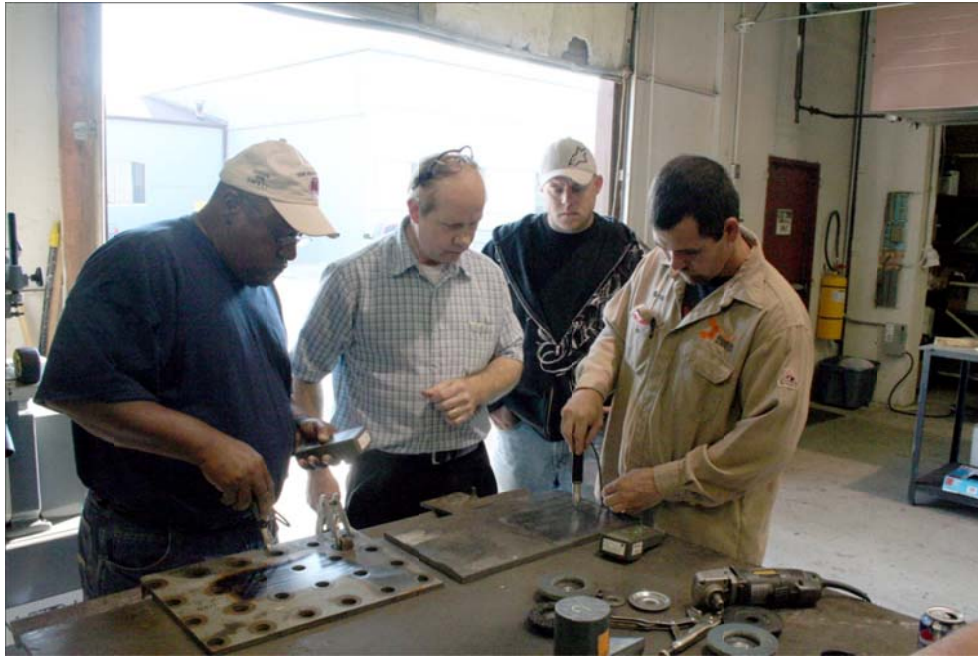
Figure 20. The HTT NDE Supervisor Teaching Mistras NDE Technicians to Perform Ultrasonic Hardness Tests at IMR.
