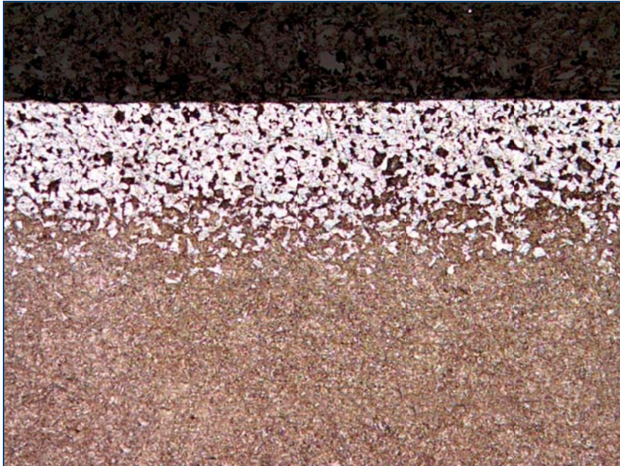
Figure 26. Surface Decarburized Layer-Cross Section from Extracted A 514 Steel Coupon Removed in Figure 24 (~100X).
