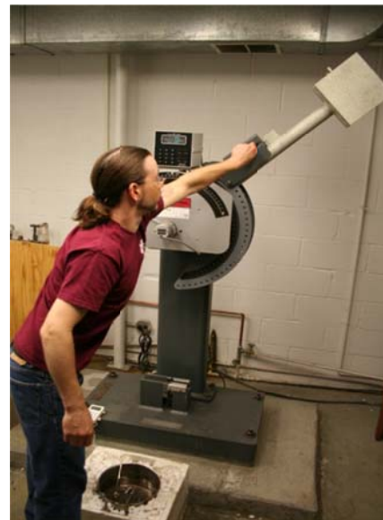
Figure 9 A. Quenching A 514 Pieces after Re-Heating (and Prior to Re-Tempering) and B. Charpy Impact Testing Re-Tempered Pieces to Investigate the Relationship between Indentation Hardness and Impact Toughness.
