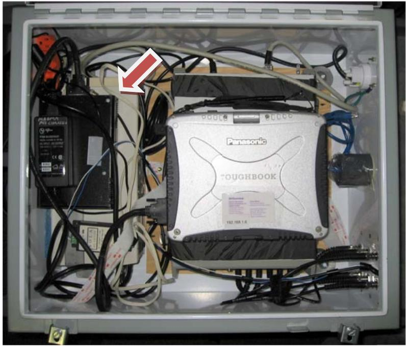
Figure 15. Battery Powered AE Monitor Mounted in Protective Case with Ruggedized Laptop PC.
