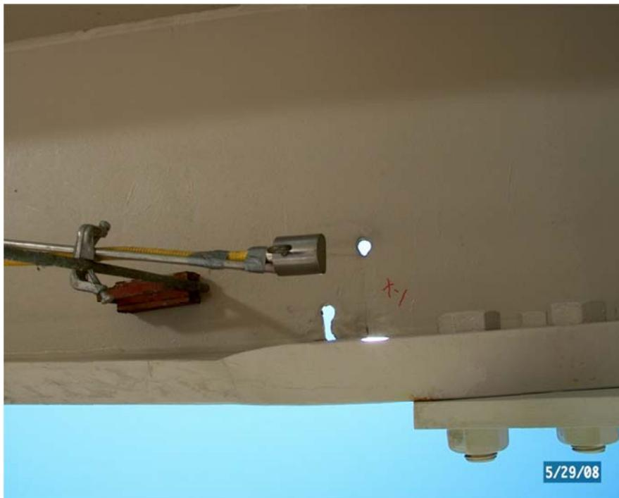
Figure 12. Upward View Showing RT Guide Tube and Collimator Aimed at 5-1/16" Crack in H beam Web for Radiograph from Underside of W
