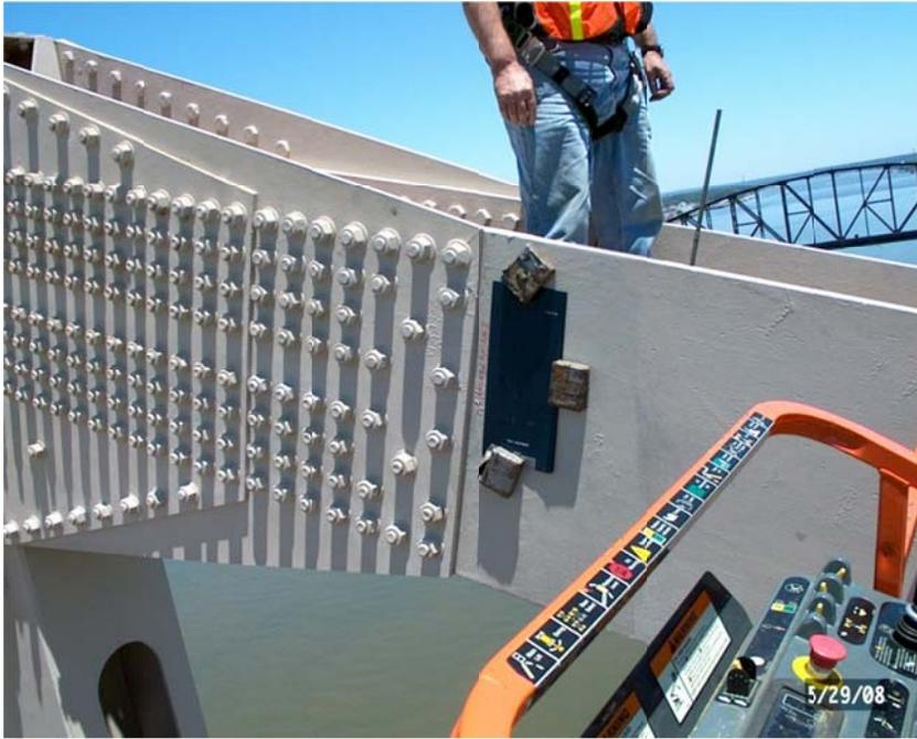
Figure 13. RT Film Pack Mounted on Outer Face of Inboard Flange for Radiograph of Flange-to-Web Fillet Weld and Flange at 5-1/16" Crack Terminus.
