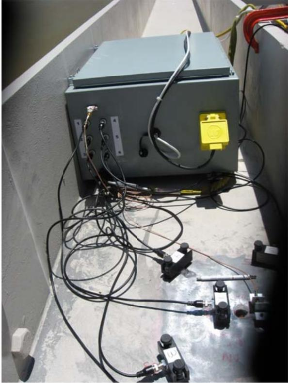
Figure 16. Transducers on H Beam Web Wired to AE Monitor Located in the Protective Case.
