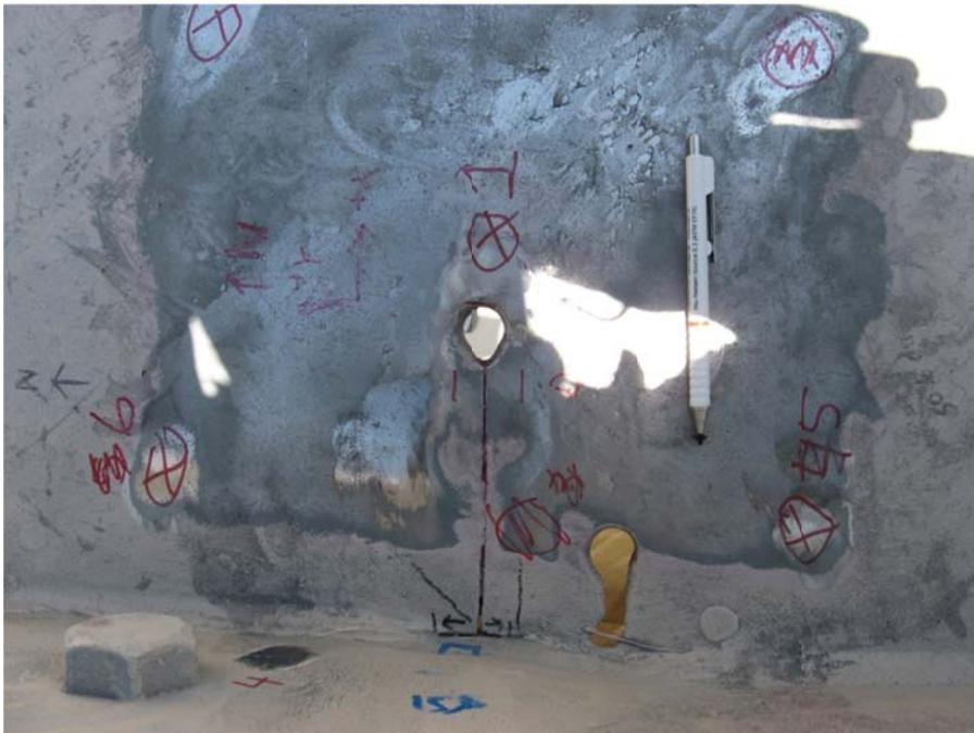
Figure 14. Upper Face of H-Beam Web (Looking Downward) Showing Layout for the Transducer Array.
