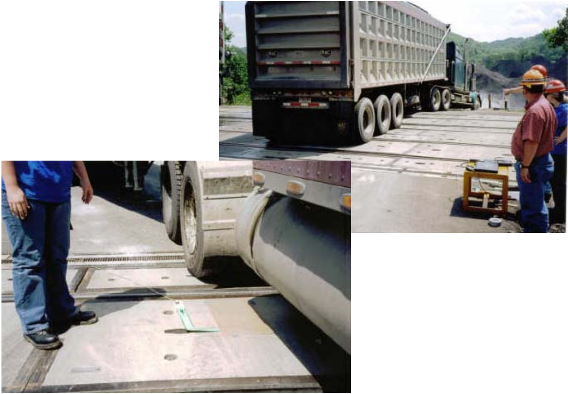
Rear Tires of Tractor of a 151,000 lb Loaded Coal Truck on Concrete Crossing of Kentucky Coal Terminal, Mile Post 6.6. May 25, 2004
