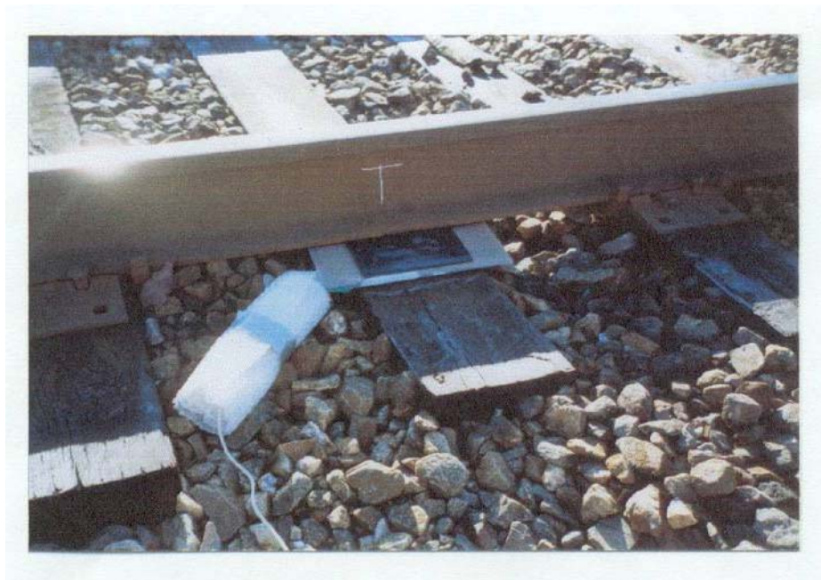
Figure 3.1c. Position of Tekscan Sensor During In-track Testing
