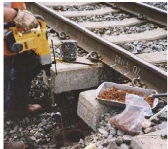
Figure 4.2 Core Drilling Operation to Obtain Asphalt Cores and Underlying Roadbed/Subgrade Samples.
