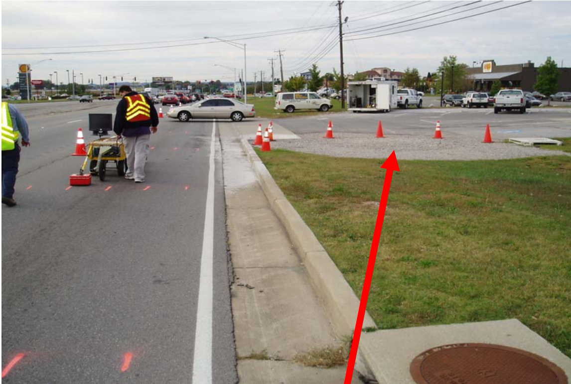
Figure 15: 200 MHz. GPR inspection
