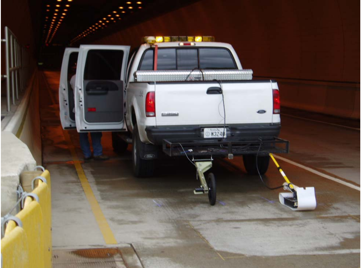
Figure 18: 900 MHz. antenna behind pick-up truck
