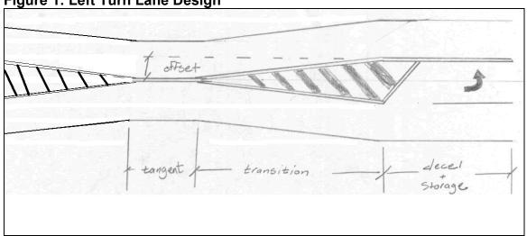
**Flush Median** - In order to provide a consistent cross section, a flush median is recommended for roadways with access point densities greater than 10 access points per mile. This density represents the approximate access spacing at which it is impossible to provide proper transitions and tangent lengths as identified in Figure 1 above. At this density a center flush median lane should be considered which can be striped as individual left turn lanes or a Two-Way Left-Turn Lane (TWLTL).
