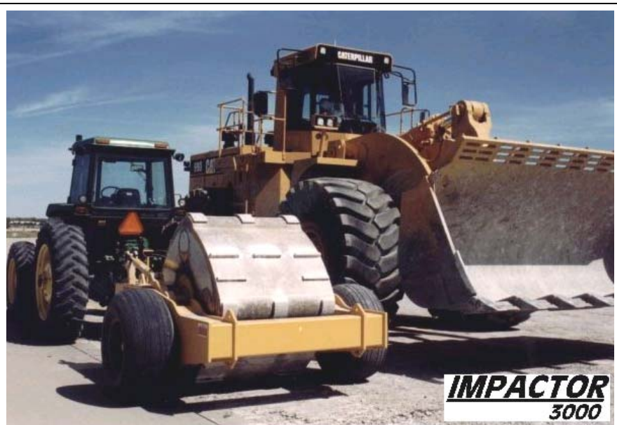
Figure 1. View of one type of non-circular impact compactor (courtesy of Impact Roller Technology(IRT)).
