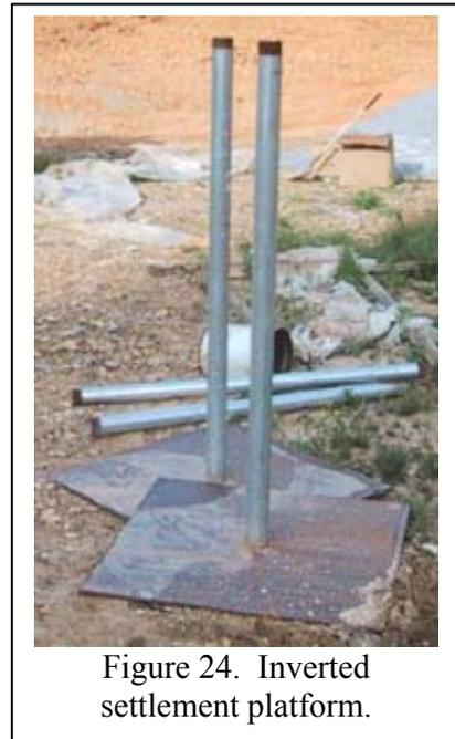
Figure 24. Inverted settlement platform.
