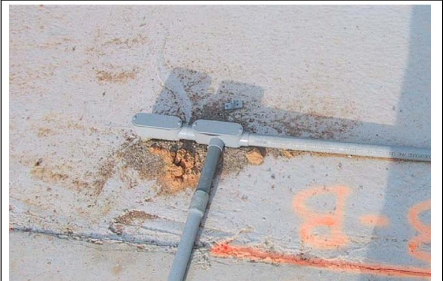
Figure 15. Strain gage wiring.
