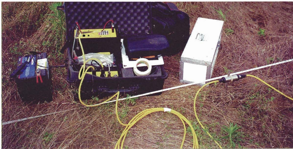
Figure 9. Field setup of the Sting/Swift multi-electrode system. Numbers refer to discussion in text.
