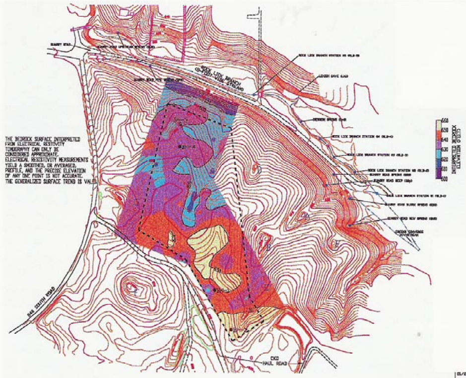
Figure 5. The generalized elevation of the bedrock surface as interpreted from Electrical Resistivity Tomography. Contour lines show the ground surface; bedrock surface elevation is color-coded.
