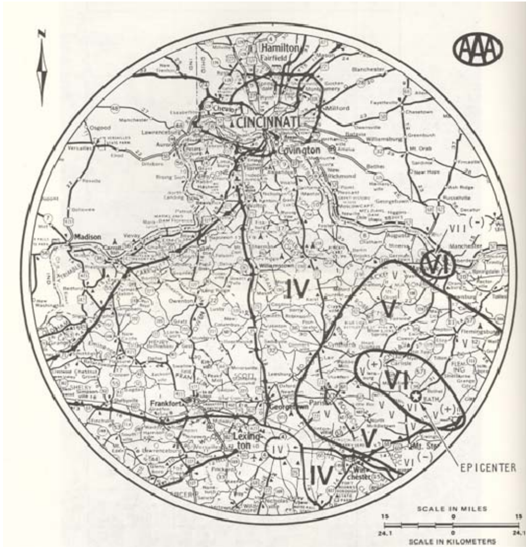
Figure 1-6. High MMI in Maysville was caused by amplified ground motion during the 1980 Sharpsburg earthquake. From Hanson and others (1980).
