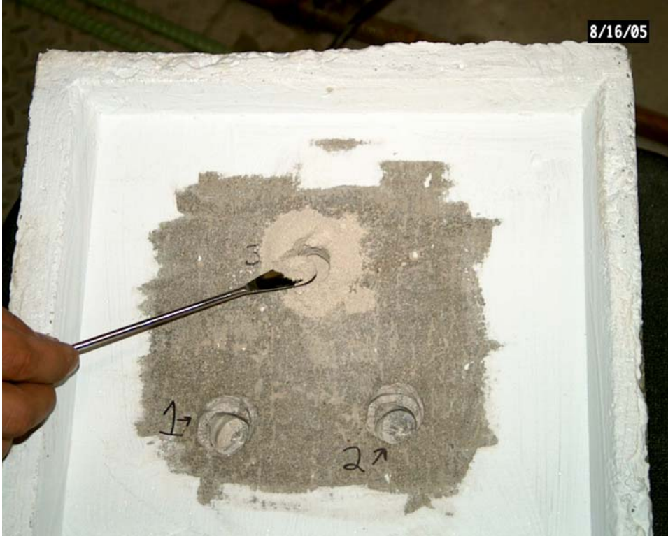
Figure 7. Sample collection for Chloride ion testing on concrete blocks
