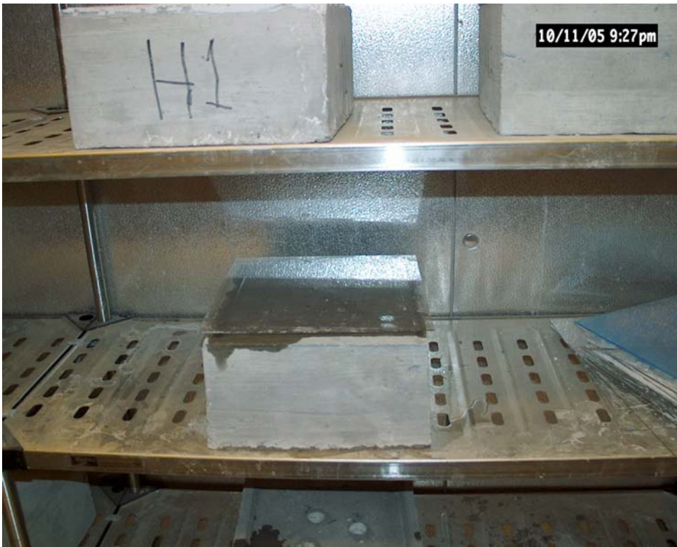
Figure 6.Ponding test with Salt Solution poured on the coated concrete blocks
