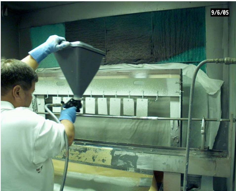
Figure 8. Applying a coating system on test panels using gravity feed spray gun
