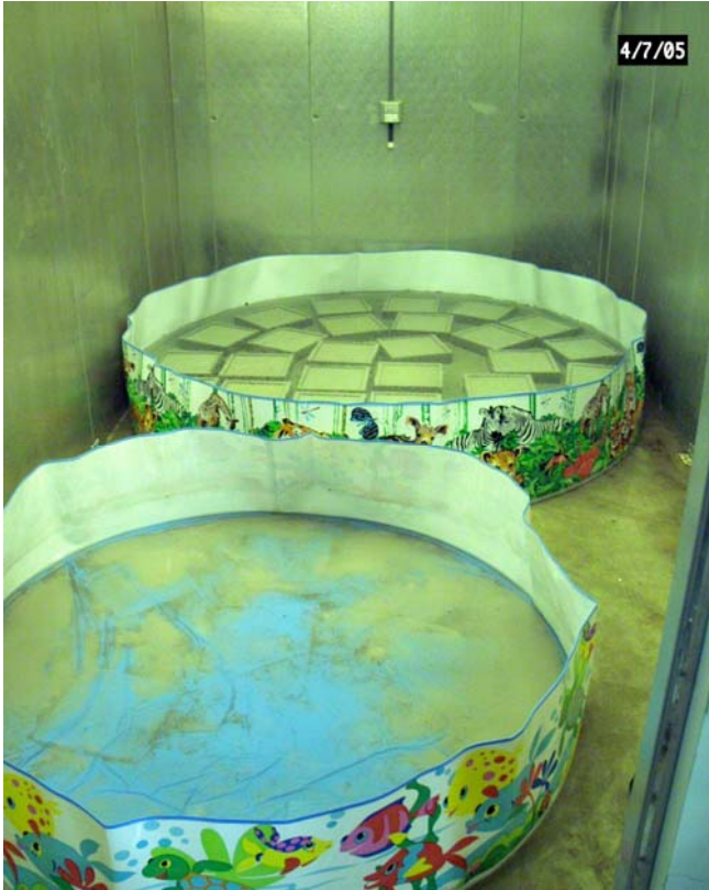
Figure 3. Concrete Blocks cured in lime water for 14 days in environmental chamber
