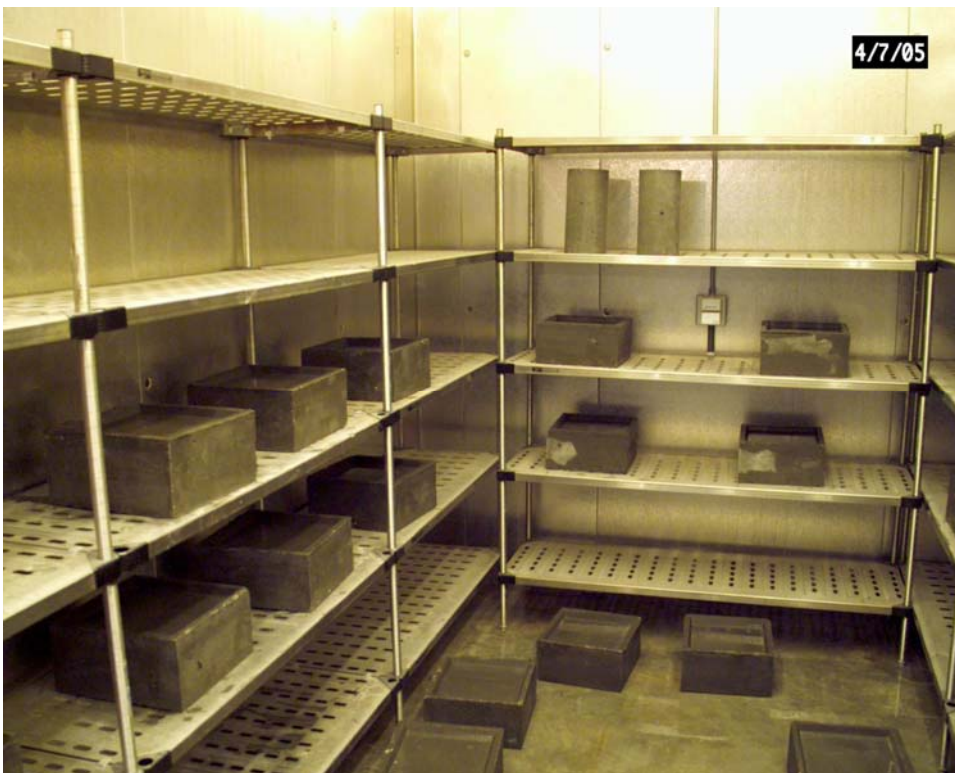
Figure 4. Concrete Blocks dried in environmental chamber for 28 days
