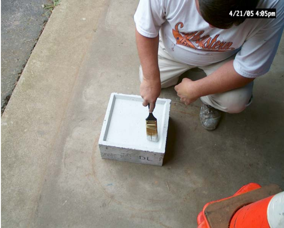
Figure 5.Coatings applied to Concrete Blocks using a brush
