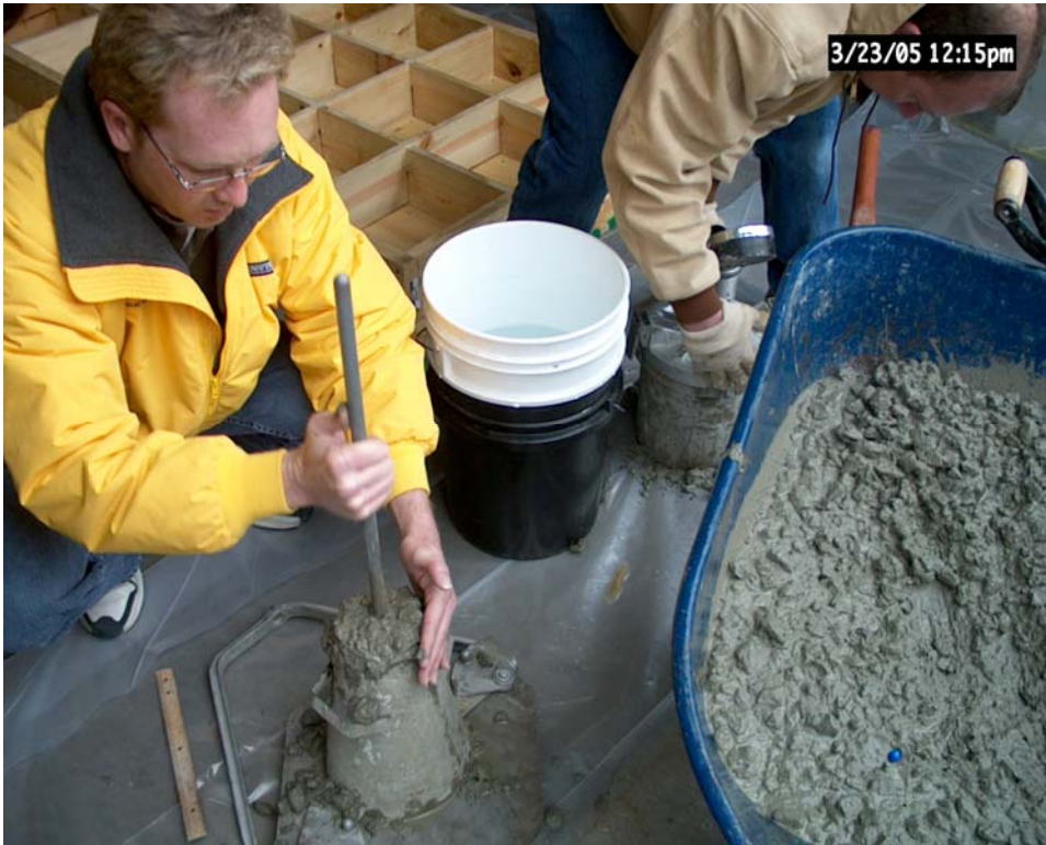
Figure 1. KYTC Division of Materials Personnel conducting Slump Test on the concrete mix at KTC
