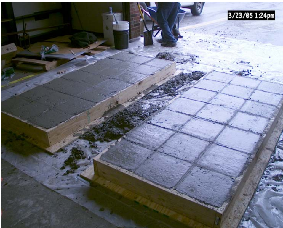
Figure 2. Finished Concrete Blocks using AA highway concrete mix
