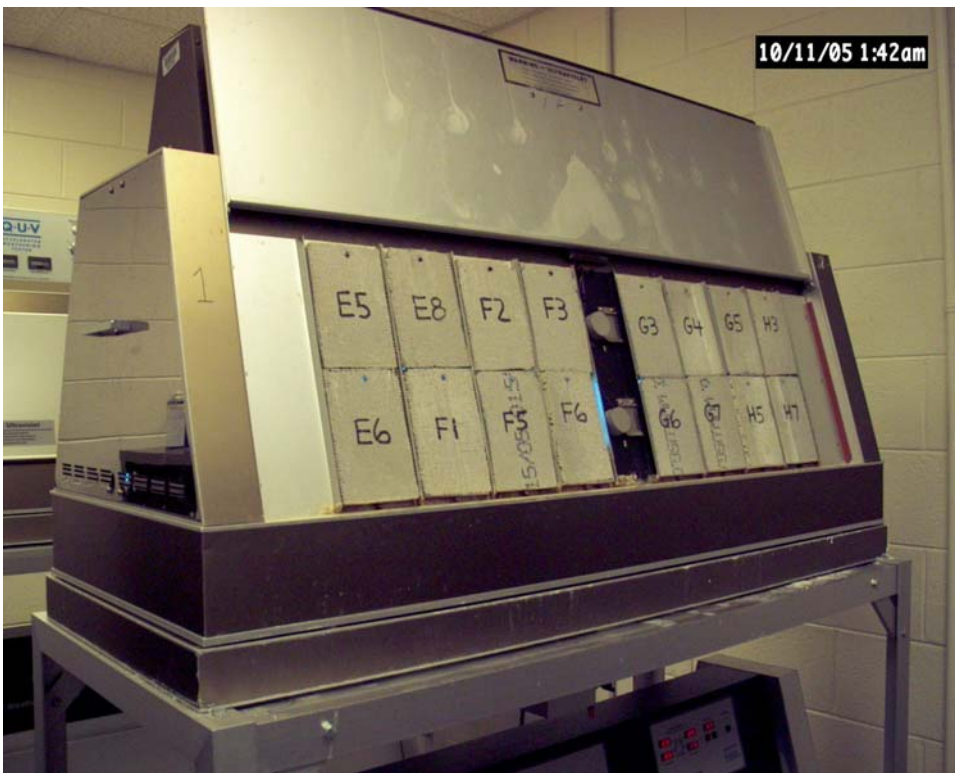
Figure 10. Test panels undergoing accelerated weathering testing in a QUV chamber
