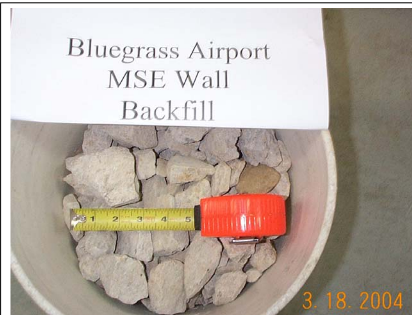
Figure 16. Backfill Sample from the MSE Wall at the Bluegrass Airport in Lexington, Kentucky.
