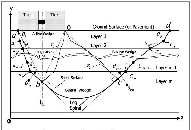
Figure 17. Method for estimating the effective value of  $N_{eff}$ .
