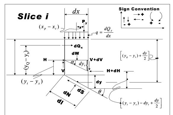
Figure 4. Forces acting on slice i.
