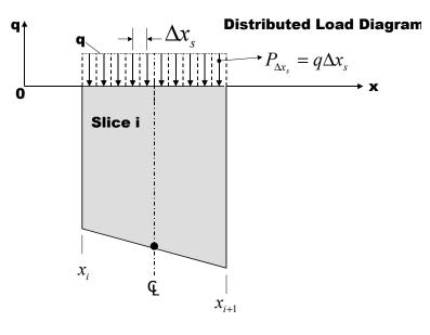
Figure 11. Scheme for treating distributed loads.
