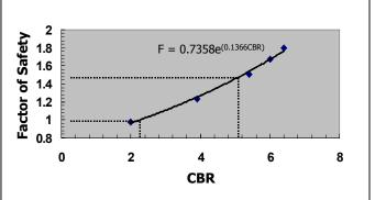
Figure 83. Factor of Safety as a function of in situ CBR, KY Route 842, Boone County.
