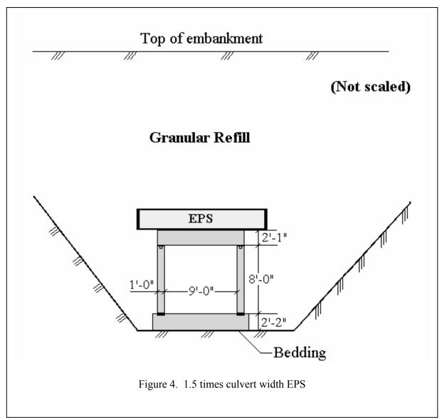
section will be a conventional one, which is used as a reference section for the other two sections with EPS. These three sections will be instrumented to measure stresses on the top and sides. Strain of the top slab will also be measured. Three "sister" reinforcing steel bars containing strain gages will be placed in the culvert during construction. Twelve earth pressure cells will be placed on the top and one side of the structure.
