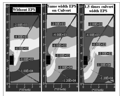
FIGURE 9. Contours of maximum principal stress with and without EPS on the top of culvert (psf)
