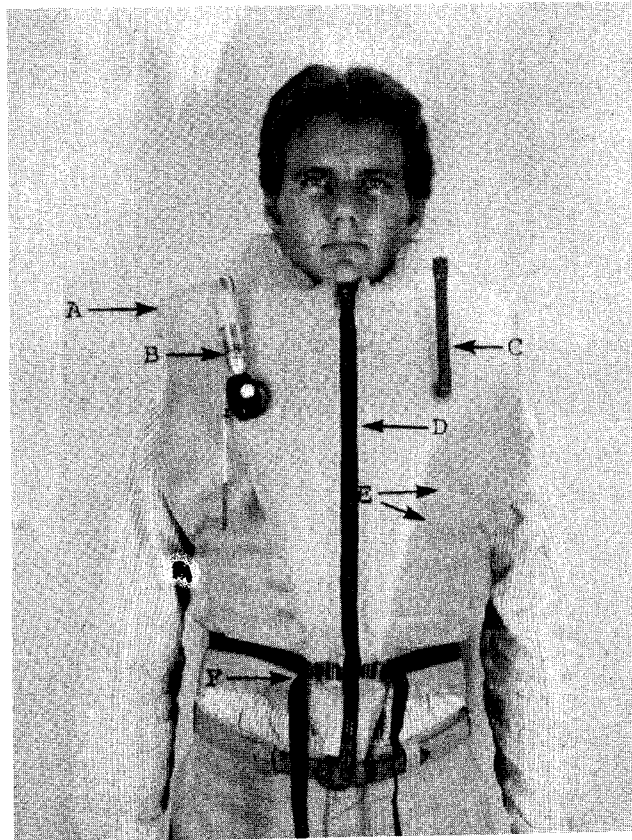
Figure 4. Prototype Life Preserver (Front View). A. Single-chamber air bladder B. One 28-g CO 2 cylinder C. Oral inflation tube D. Front zipper E. Heat-sealed areas F. Belt
