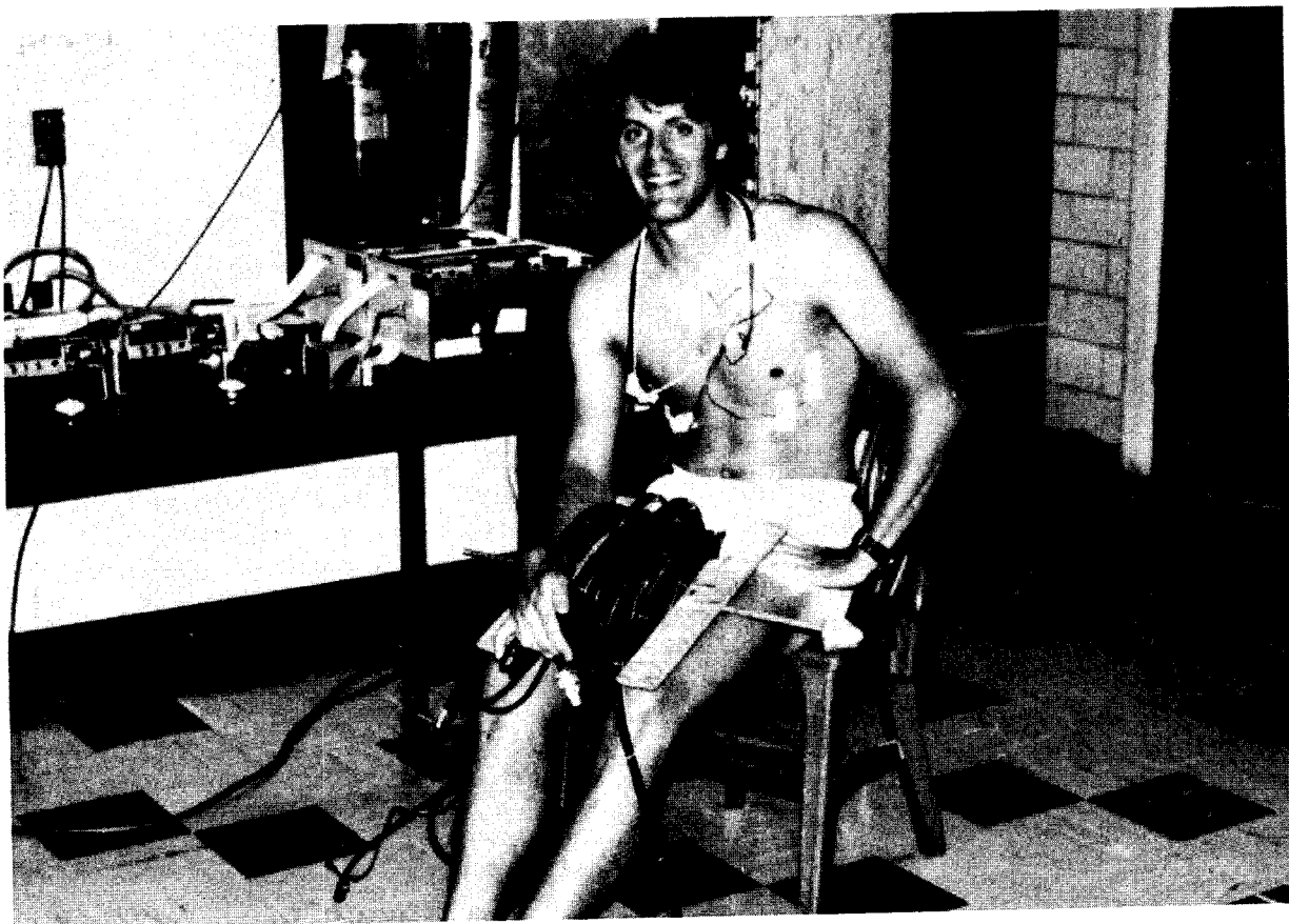
Figure 8. Subject instrumented with adhesive chest electrodes.
