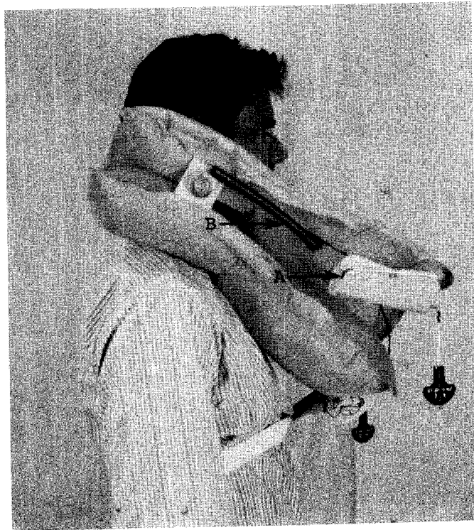
Figure 2. Standard Personal Flotation Device (Side View). A. 16-g CO 2 cylinder B. Oral inflation tube
