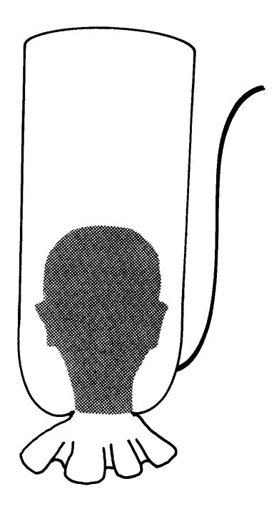
Figure 3. Sheldahl hood modified to include a continuous-flow gas inlet.
