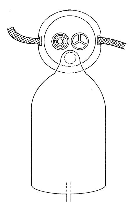
Figure 6. Front view of unmodified Scott-Sierra passenger mask.
