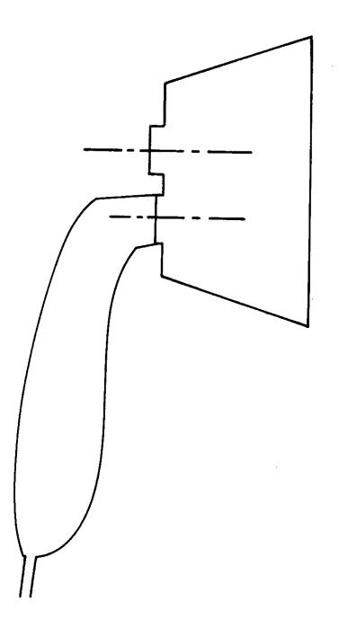
Figure 7. Side view of unmodified Scott-Sierra passenger mask.
