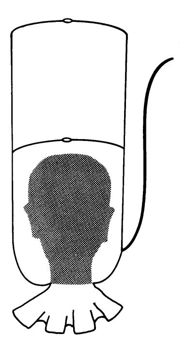
Figure 5. Sheldahl hood modified to include a dual compartment system.
