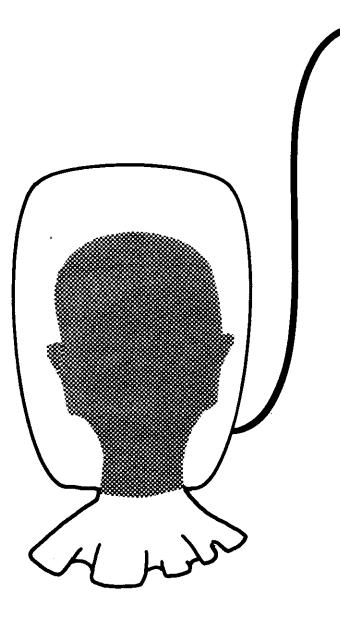
Figure 4. Sheldahl hood modified by reduction of the internal volume.
