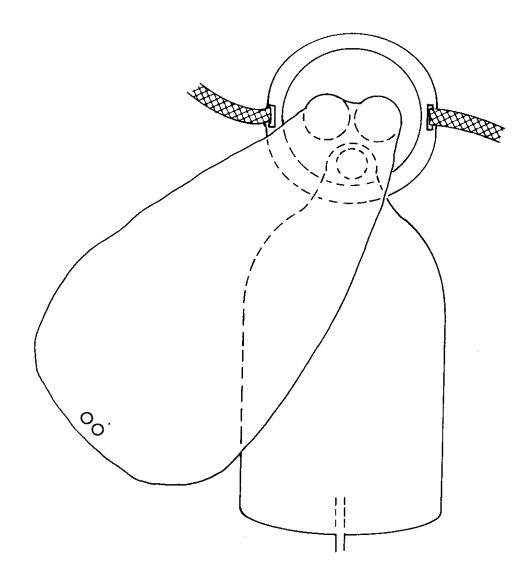
Figure 8. Front view of modified Scott-Sierra passenger mask.
