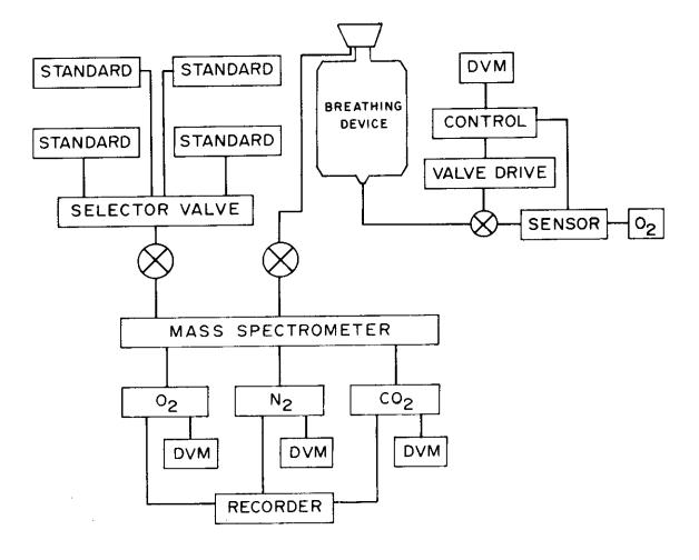
Figure 1. Diagram of the system used for testing protective breathing devices.
