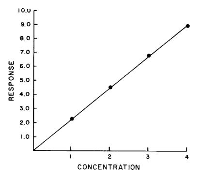
FIGURE 4. Analytical response vs. pentane concentration.
