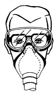
FIGURE 9. Goggles with venting tubes positioned under mask lip.
