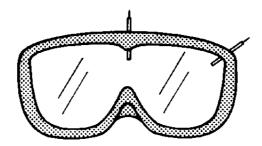
FIGURE 1. Location of the sample needles in goggles.
