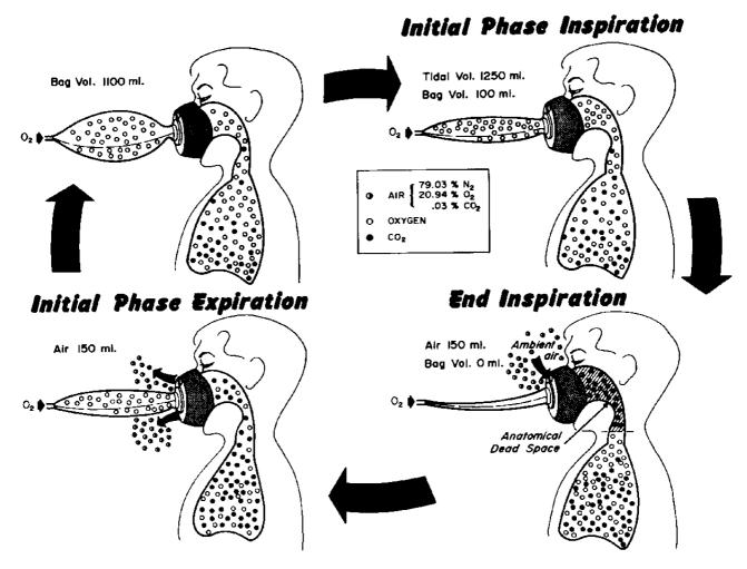
FIGURE 3. Diagrammatic representation of the sequential performance of a phase dilution passenger oxygen mask.
