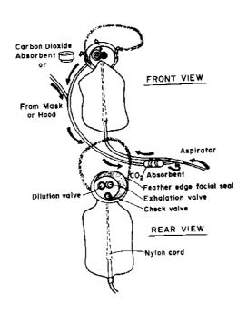
FIGURE 5. Two alternative concepts in modifying a passenger oxygen mask to provide respiratory protection from smoke and toxic gas. A third improved variation has been constructed that uses a carbon dioxide absorbent bed superimposed between the exhalation and dilution valves and an additional reservoir, thereby producing a double pass of the exhaled gases through the absorbent bed.
