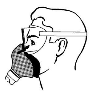
FIGURE 5. Mask leakage along masal bridge.
