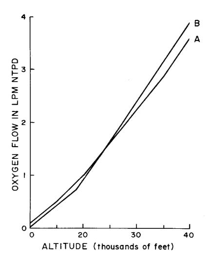
FIGURE 2. (A) Minimum passenger oxygen flow as required by the Federal Aviation Regulations, (B) hypothetical curve provided by manufacturer to meet the requirements.
