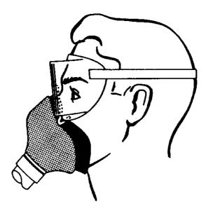
FIGURE 8. Goggles with short venting tubes.
