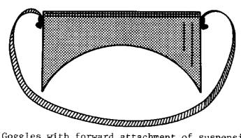
FIGURE 7. Goggles with forward attachment of suspension strap.
