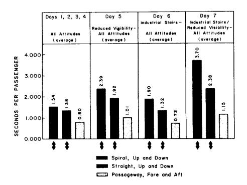
FIGURE 8. Comparison of passenger flow on all test equipment.
