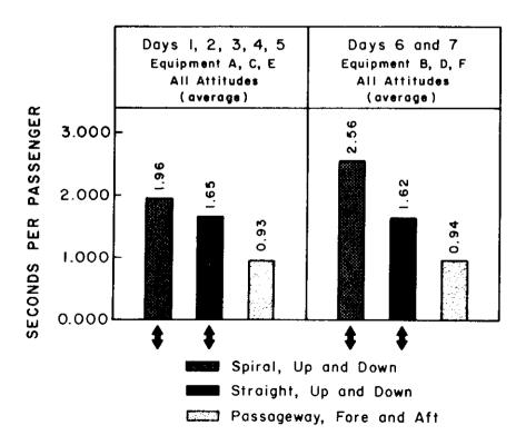
FIGURE 10. Comparison of passenger flow rates.
