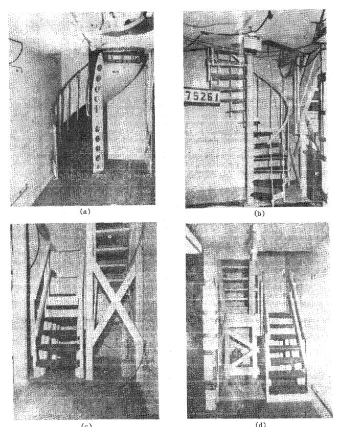
FIGURE 1. Stairways used in Phase II tests: (a) spiral stairway similar to that used between decks of a Boeing 747; (b) industrial spiral stairway; (c) right-ascending turn, straight-segmented stairway; and (d) left-ascending turn, straight-segmented stairway.
