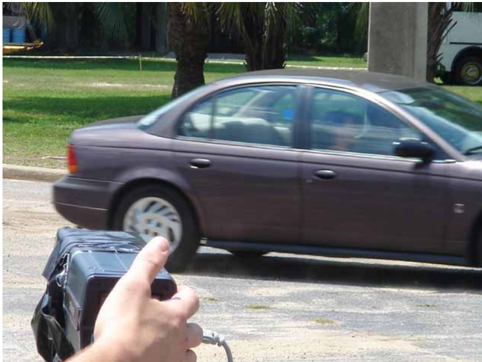
Researchers measure vehicle speed to help determine sign comprehension distances in human factors studies.
