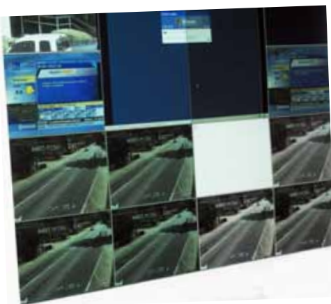
Above: The video wall enables TERL to simulate a Transportation Management Center.
