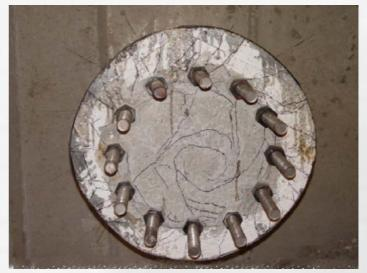
The face of this test shaft illustrates the yielding of bolts, breakout cracks around perimeter, and torsion cracks in center.
