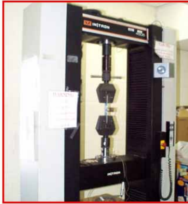
Figure 40. Photo. Typical tension test setup.
