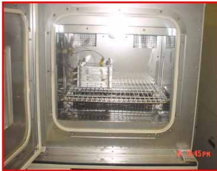
Figure 42. Photo. Freeze-thaw chamber.
