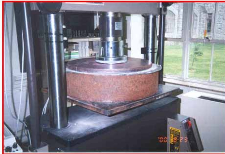
Figure 238. Photo. VT pushout test setup.
