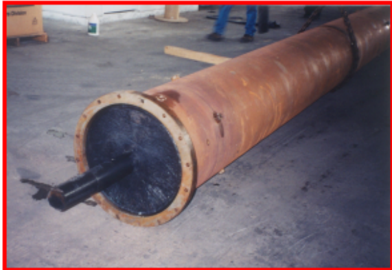
d) Finished pile ready to be extruded from mold
