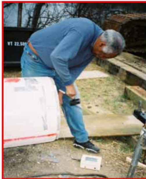
b) PIT on FRP pile before installation
