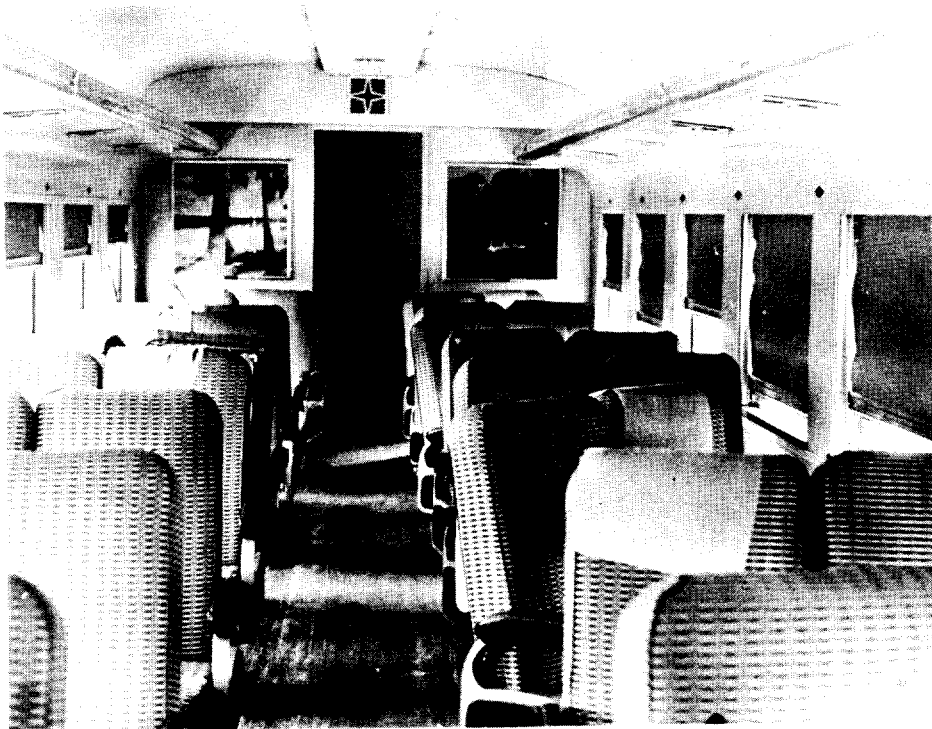
FIGURE 21. Passenger Cars 6, 7, 8, and 9 did not overturn and Passenger Car No. 6 is shown here to depict relatively minor damage to these cars.
