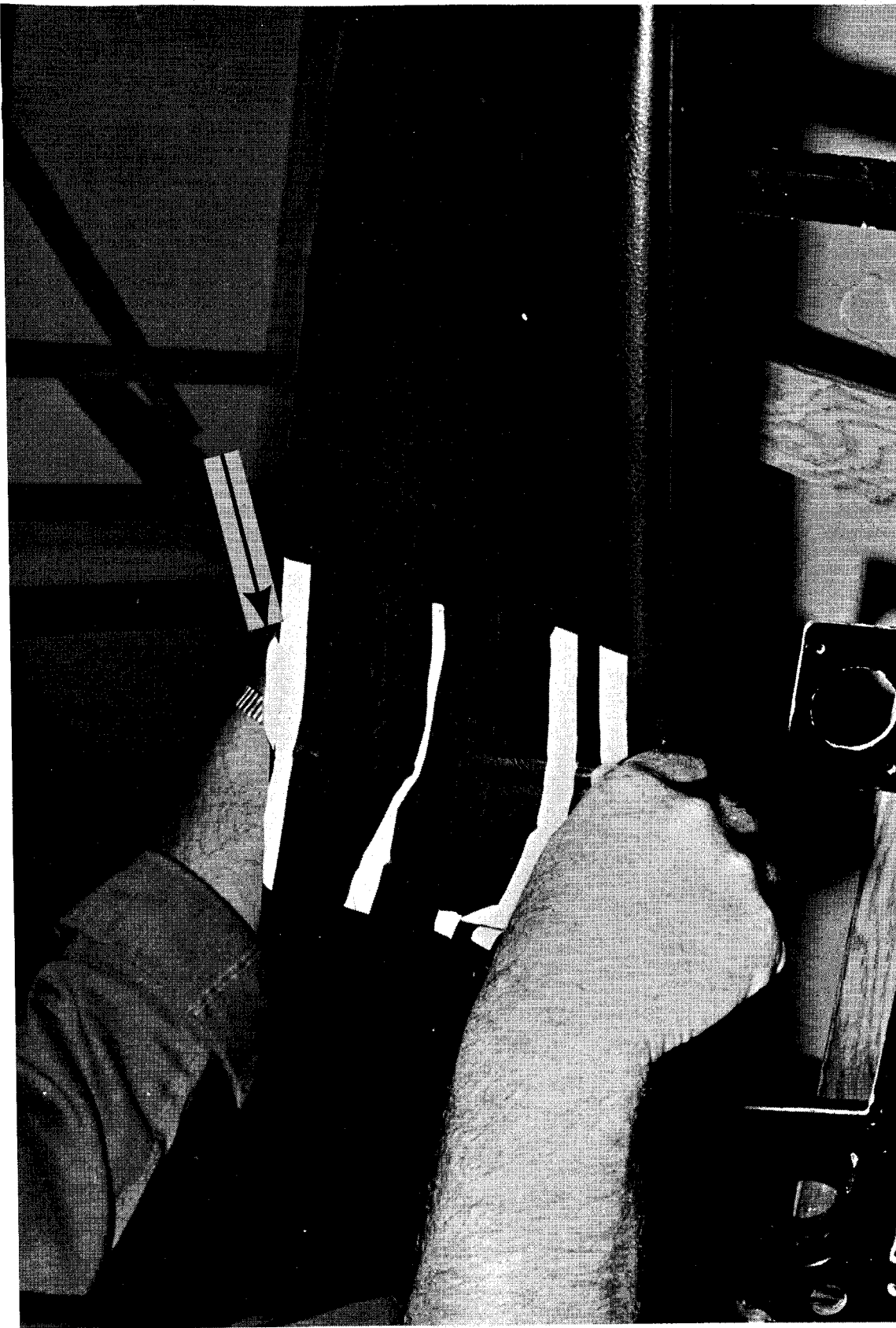
FIGURE 5. Broken edge of fiberglass cut through thin padding (note arrow).
