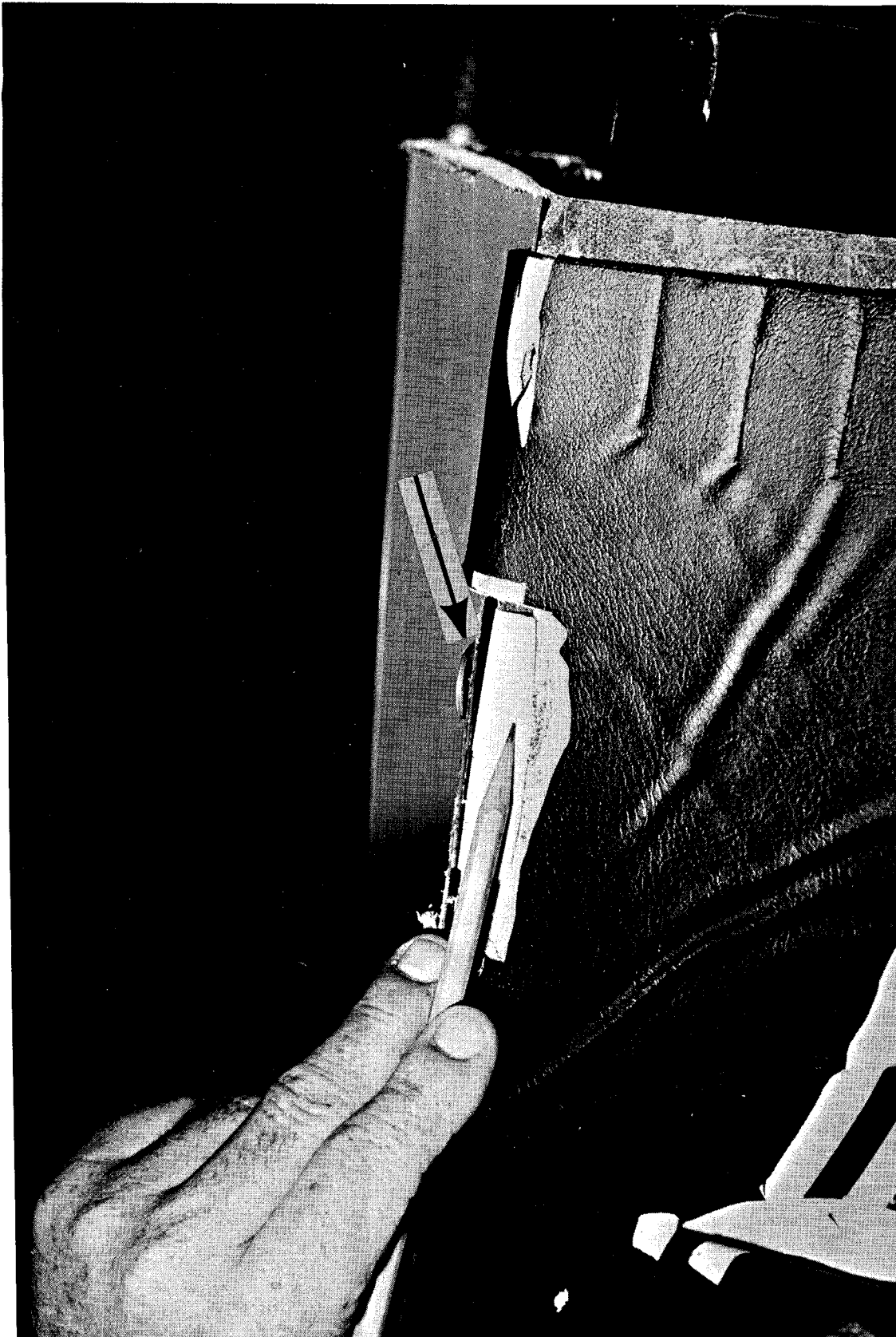
FIGURE 7. Fiberglass edge at break (see arrow). Dime is shown for thickness reference.
