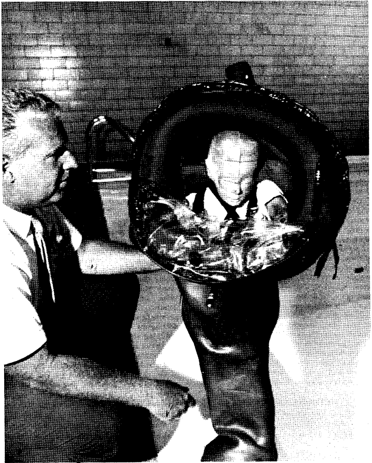
FIGURE 1. Initial prototype of the infant flotation device occupied by a child anthropomorphic dummy.
