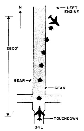
FIGURE 16. Skid path and final location of Salt Lake City 727.
