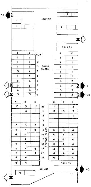
FIGURE 12. Diagram of exit utilization in Denver DC-8 evacuation. Numerals in seats are keyed to exit numbers. Figures adjacent to exits denote total number of passengers using the exit.
