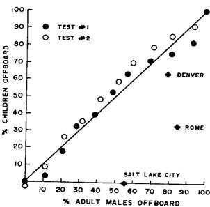
Figure 40.a.b. Cumulative percentage of adult females (upper figure) and children (lower figure) evacuated as a function of adult males evacuated in SST evacuation tests. The inset points represent corresponding percentages in the three accidents.
