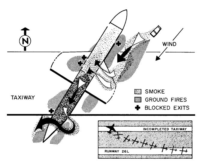
FIGURE 1. Path (inset) and final position of Denver DC-8. Smoke from ground fuel fires forward of right wing entered cabin through opened right window exits. Concentration of smoke was particularly intense in 2nd-class (aft) passenger compartment due to draft produced by open right rear galley exit.
