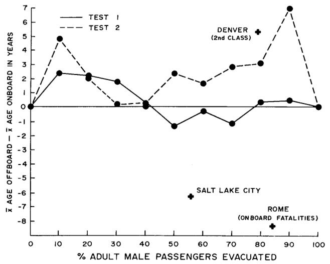
FIGURE 41. Difference in mean age of onboard and offboard males plotted against total passengers deplaned for evacuation tests and accidents.
