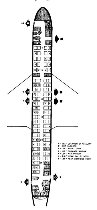
FIGURE 28. Pattern of exit utilization by passengers of the Rome 707.
