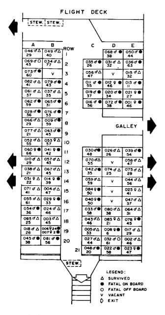
Figure 18. Seating diagram (non-scale) of Salt Lake City 727 showing distribution of passengers, their sex, survival status, age (2 digit numeral), and identification number (3 digit numeral) based on alphabetical listing by passenger surname.
