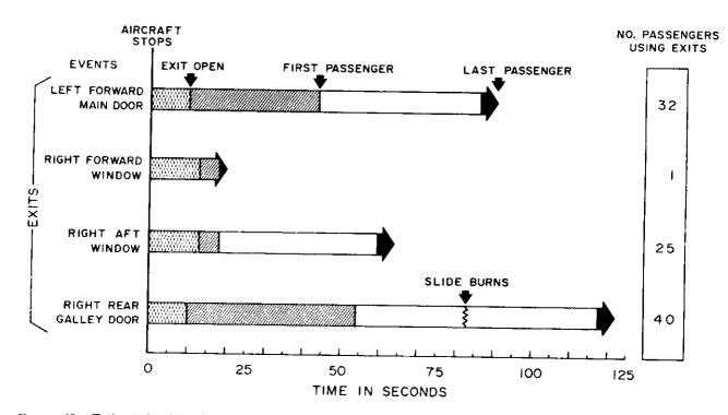
FIGURE 13. Estimated minimal evacuation times for exits used in Denver DC-8 crash. Time estimates are derived from AIA evacuation analysis of DC-8 test evacuation except at aft door where a 10 sec. delay is added for slide deployment and a rate of 2 sec./passenger assumed after the slide burned.
