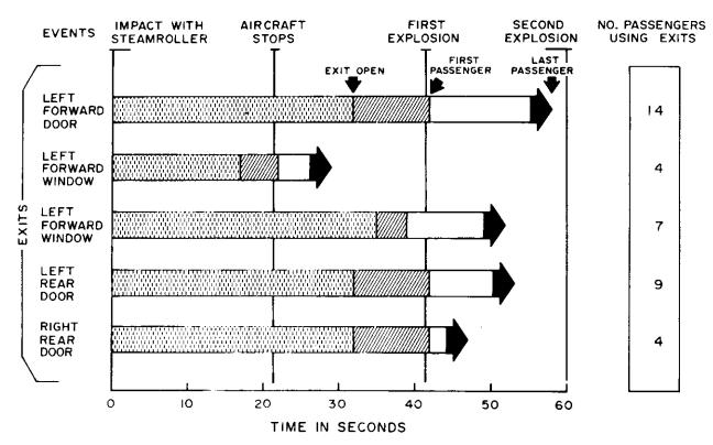
FIGURE 29. Evacuation sequence of Rome 707 showing approximate escape times and number of escapees from each exit.
