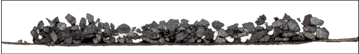
Figure 6-1 Cross-section of the triple seal specimen after MMLS3 loading
