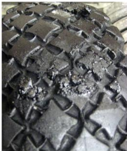
Figure 5-2 Double seal specimen with CRS-2 emulsion and MMLS3 tire after bleeding: (a) double seal specimen using CRS-2 emulsion; (b) tire with aggregate
