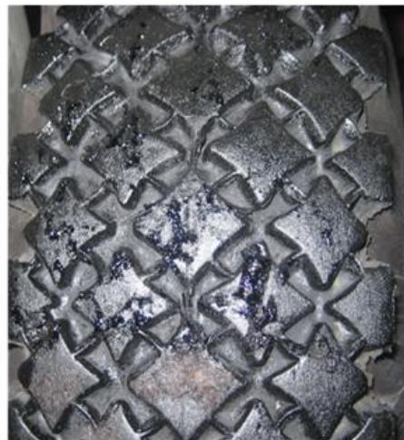
Figure 5-2 Double seal specimen with CRS-2 emulsion and MMLS3 tire after bleeding: (a) double seal specimen using CRS-2 emulsion; (b) tire with aggregate
